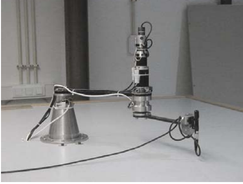
Figure 6: : Experimental Setup, Planar Robotic Manipulator with eye-in-hand, camera looking up.
