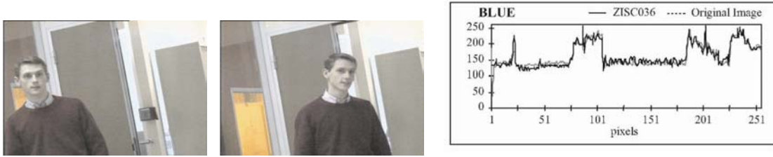
Figure 10: Result concerning movie coloration showing from left to right the image used to train the neural network and the result obtained on coloration of an unlearned scene (left). Blue component cross sections comparison between the coloured (reconstructed) and the original images in generalization phase (right).
