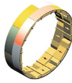
Figure 4: Two consecutive rings of the formwork. Each ring consists of eight segments.
