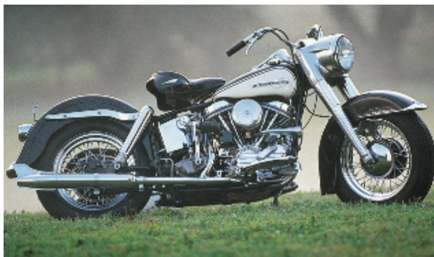
FIGURE 12.16 Chromium plating lends decorative flair as well as electrochemical protection to the steel of this motorcycle. Large quantities of electricity are needed for chromium plating because six electrons are required to produce each atom of chromium from chromium(VI) oxide.
