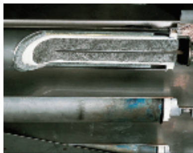
FIGURE 12.23 A sodium–sulfur battery used in an electric vehicle.
