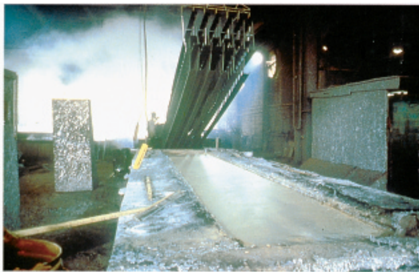
FIGURE 12.19 Steel girders are galvanized by immersion in a bath of molten zinc.
