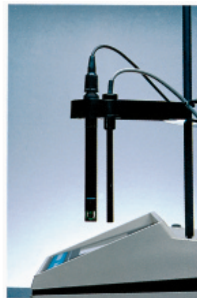
FIGURE 12.11 A glass electrode in a protective plastic sleeve (left) is used to measure pH. It is used in conjunction with a calomel electrode (right) in pH meters such as this one.
