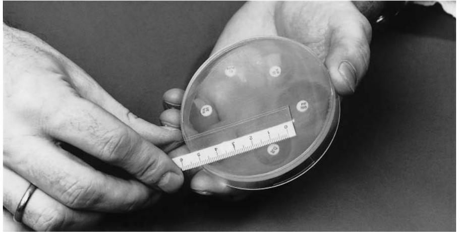
If the medium is opaque, the zone can be measured by means of a pair of calipers.
