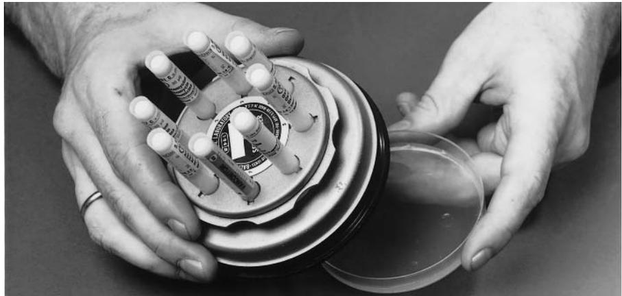
A maximum of seven discs can be placed on a 9–10 cm plate. Six discs may be spaced evenly, approximately 15 mm from the edge of the plate, and 1 disc placed in the centre of the plate. Each disc should be gently pressed down to ensure even contact with the medium.
