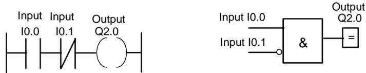
Figure 5.29 Ladder diagram and equivalent function block diagram
