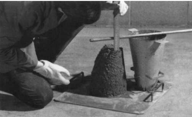
Figure 38: Measuring the slump of concrete.
