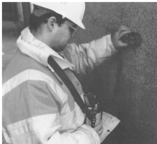
Figure 46: Using the covermeter to estimate the depth and direction of the reinforcement in a structure.
