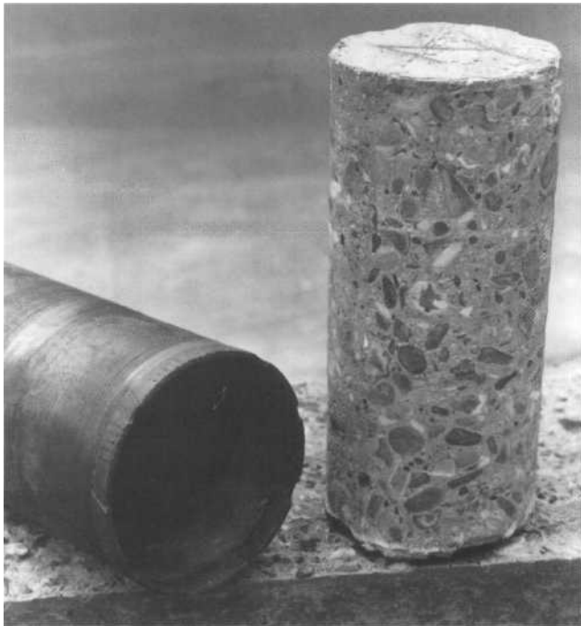
Figure 42: As well as providing a specimen for strength testing, the core gives a good indication of the distribution of the aggregate and the degree of compaction.
