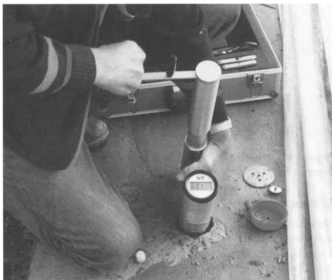
Figure 45: Measuring the force required to pull out an insert cast into a floor.
