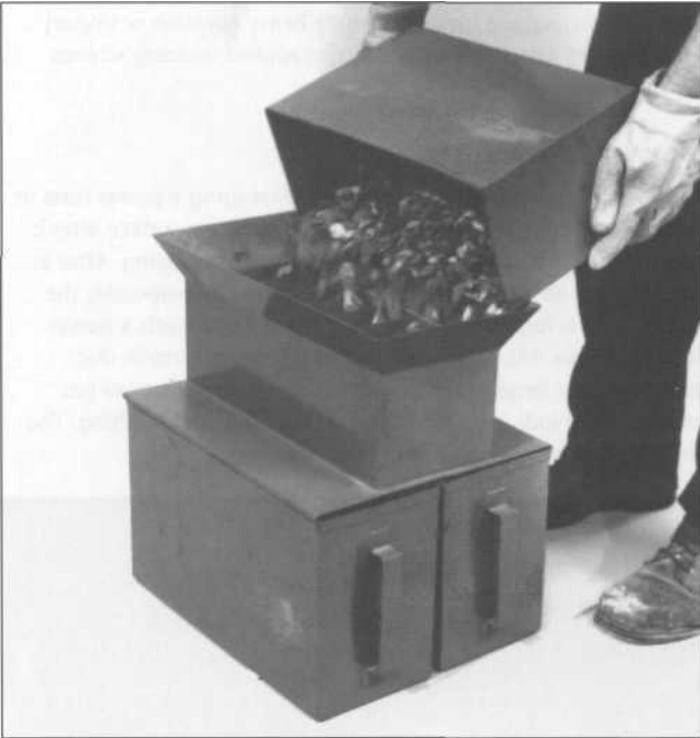
Figure 34: Dividing a sample of aggregate with a riffle box.
