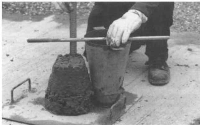
Figure 5: A typical S2 consistence class concrete with a cement content of 300 kg/m 3 .
