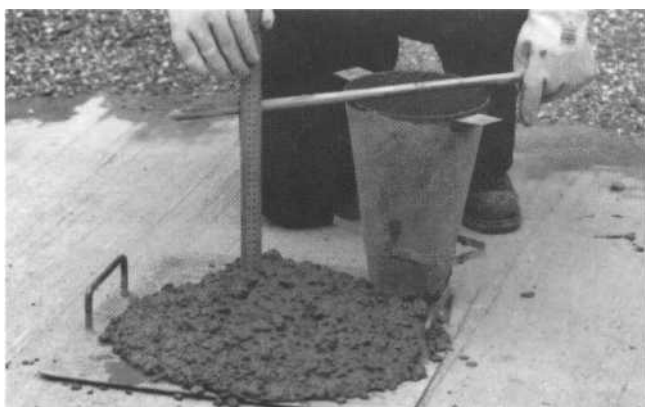
Figure 6: A similar concrete to that shown in Figure 5, but after the addition of a superplasticizer.
