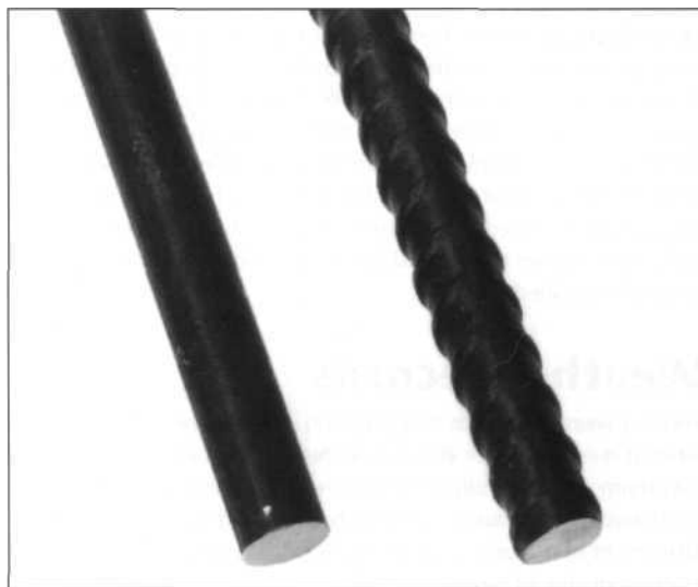
Figure 25: Types of reinforcement in general use: plain mild steel bar (left); high yield bar (right).
