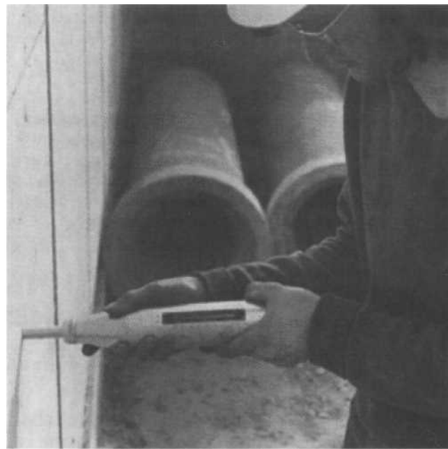
Figure 43: Measuring the surface hardness of concrete with a Schmidt hammer.
