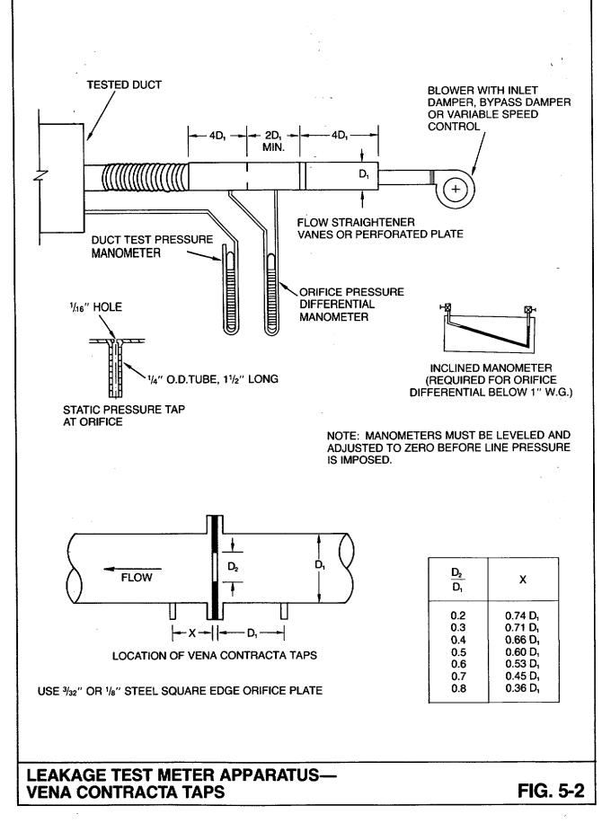
5.14 Airflow across a sharp edge orifice with standard air density of .075 #/ft<sup>3</sup> is calculated from
