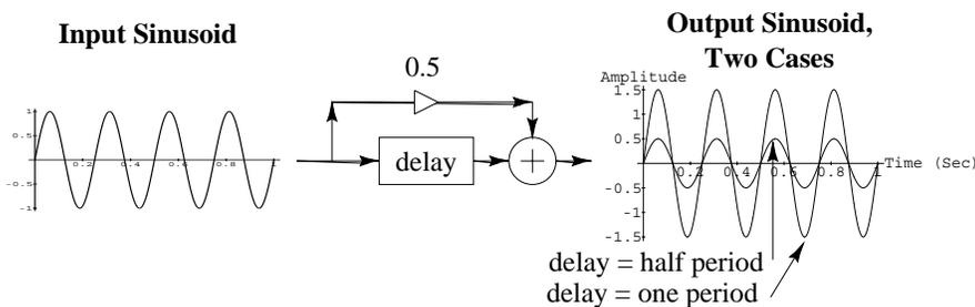
Figure 5.3: A comb filter with a sinusoidal input.
