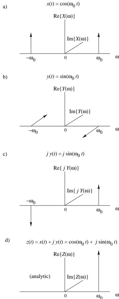
Figure 5.8: Creation of the analytic signal  $z(t) = e^{j\omega_0 t}$  from the real sinusoid  $x(t) = \cos(\omega_0 t)$  and the derived phase-quadrature sinusoid  $y(t) = \sin(\omega_0 t)$ , viewed in the frequency domain. a) Spectrum of  $x$ . b) Spectrum of  $y$ . c) Spectrum of  $jy$ . d) Spectrum of  $z = x + jy$ .
