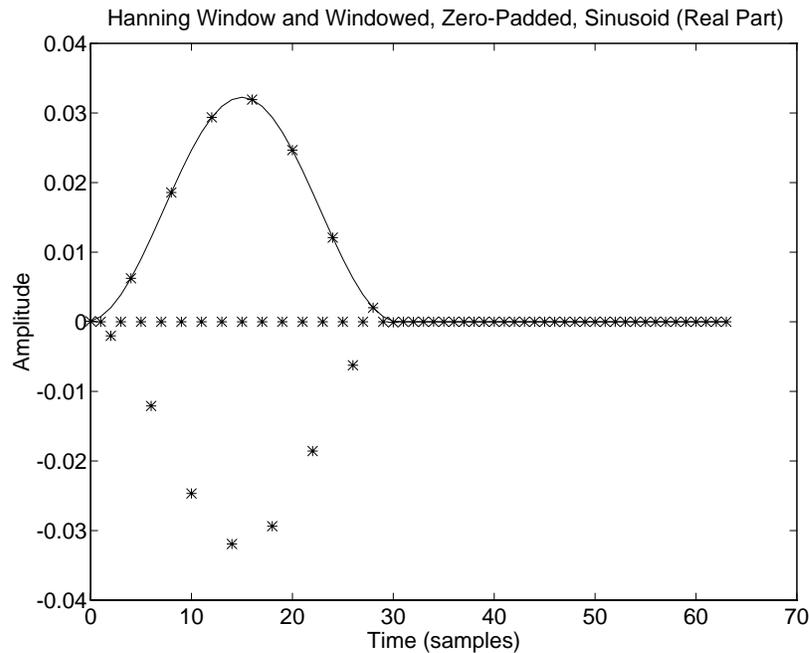
Figure 9.7: A length 31 Hanning Window (“Raised Cosine”) and the windowed sinusoid created using it. Zero-padding is also shown. The sampled sinusoid is plotted with ‘\*’ using no connecting lines. You must now imagine the continuous sinusoid threading through the asterisks.
