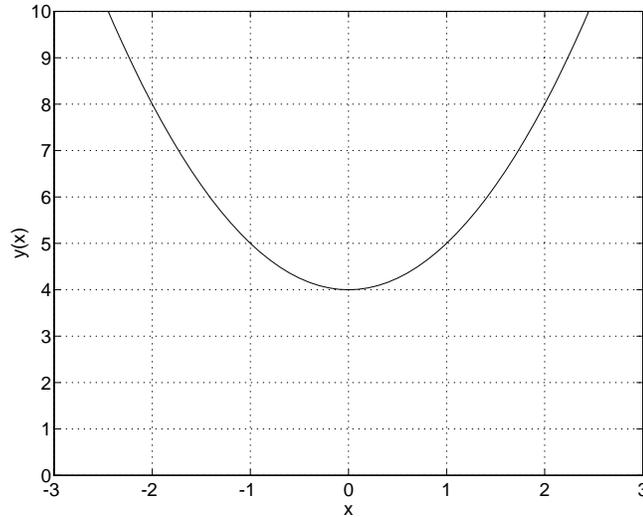
Figure 2.1: An example parabola defined by  $p(x) = x^2 + 4$ .
