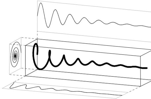
Figure 5.9: Exponentially decaying complex sinusoid and its projections.
