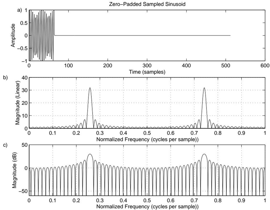
Figure 9.4: Zero-Padded Sinusoid at Frequency  $f = 0.25 + 0.5/N$ .
