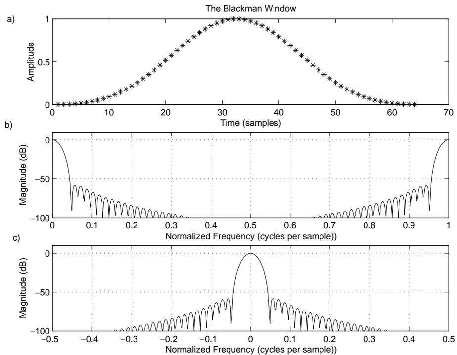
Figure 9.5: The Blackman Window. a) The window itself in the time domain. b) DB Magnitude spectrum of the Blackman window. c) Blackman-window DB magnitude spectrum plotted over frequencies  $[-0.5, 0.5]$ .
