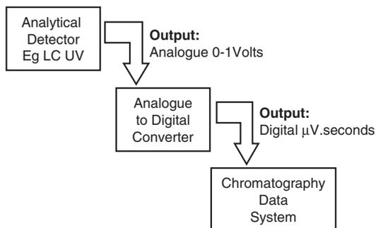
**Figure 2.6-1:** Typical A/D conversion of chromatography signals.
