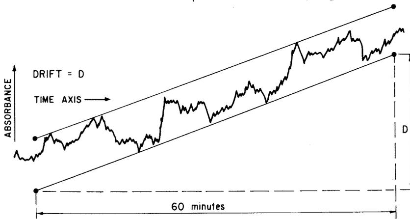
Figure 2.6-5: ASTM noise and drift measurements for LC UV detectors ([115]).
