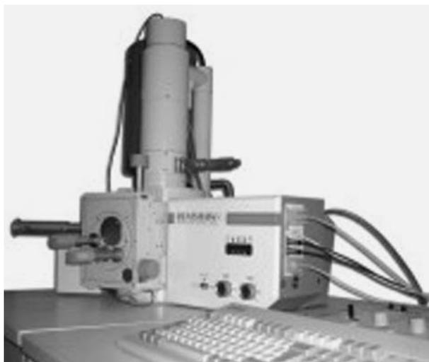
**Figure 7.5.** A combined SEM/Raman system. The Raman spectrometer is integrated into the side of the SEM. (Reproduced with permission from Renishaw plc.)
