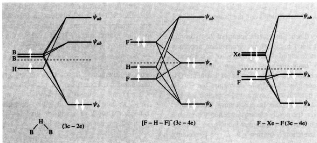
**Figure 3.11** Schematic representation of the energy levels in various types of 3-centre bond. The B-H-B (“electron deficient”) bond is non-linear, the (“electron excess”) F-Xe-F bond is linear, and the A-H...B hydrogen bond can be either linear or non-linear depending on the compound.
