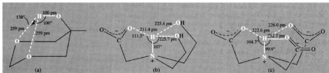
**Figure 3.5** Some examples of branched H bonds: (a) the bifurcated bond in 1,3-dioxanol-5<sup>(49)</sup>; and trifurcated bonds in (b) *N,N*-bis(2-hydroxyethyl)glycine<sup>(50)</sup> and (c) the nitrilotriacetate dianion.<sup>(51)</sup>
