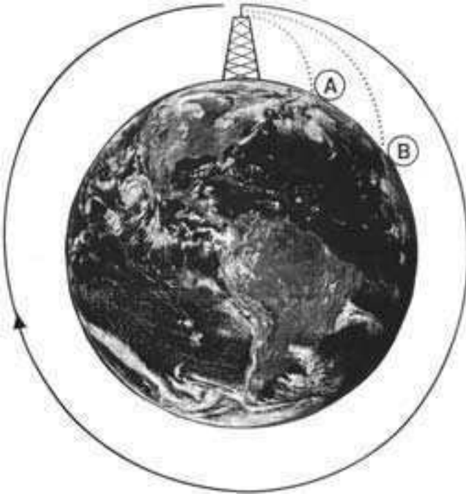
Figure 4.9 Sir Isaac Newton studied the motion of a satellite around its parent body by first imagining the behavior of a cannonball fired from a cannon in the horizontal direction, when that cannon was placed and securely attached to a very tall tower or mountain. As the muzzle velocity of the cannonball increased, it would fall to Earth farther and farther away from the tower until it reached a sufficient velocity (called the orbital velocity) that it could actually travel all the way around Earth without ever falling to the ground. NASA image modified by author.
