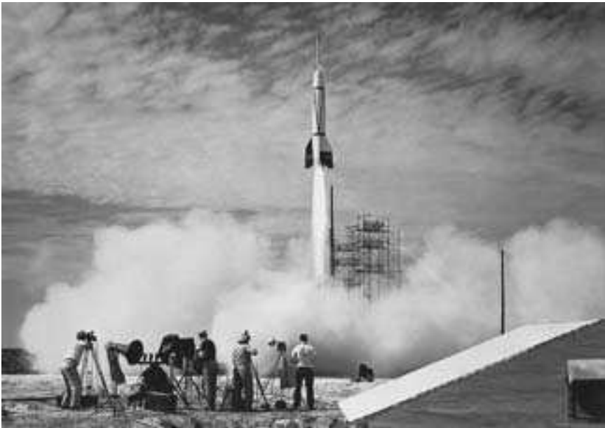
The Bumper 8, a modified, captured German V-2 rocket, was the first rocket launched from Cape Canaveral, Florida (July 24, 1950). Image courtesy of NASA.
