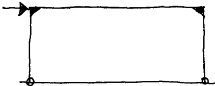
2 PIN JOINTS & 2 STIFF JOINTS
