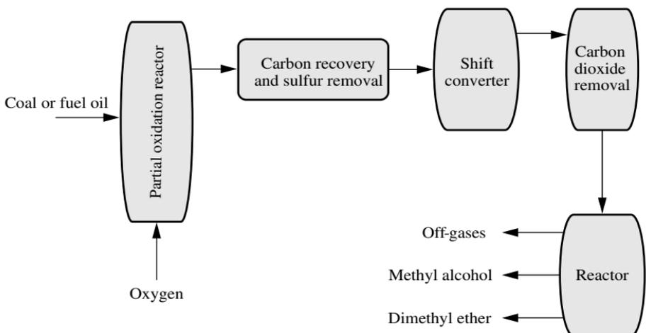
FIGURE 1 Manufacture of methyl alcohol from synthesis gas.
