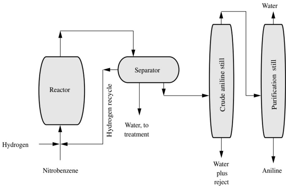
FIGURE 2 Vapor phase reduction of nitrobenzene to aniline.
