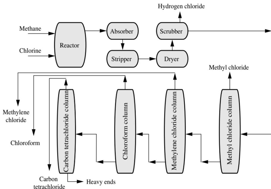
FIGURE 1 Production of chloromethanes by chlorination of methane.
