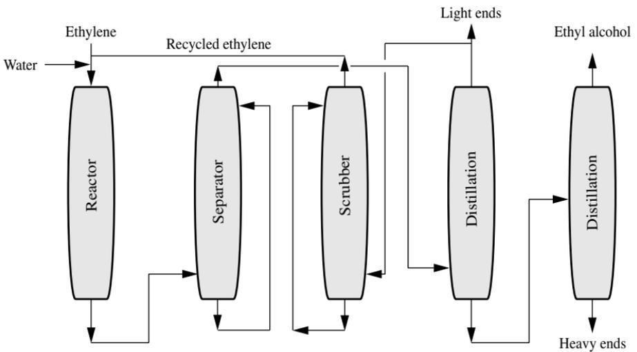
**FIGURE 2** Manufacture of ethyl alcohol by direct hydration.
