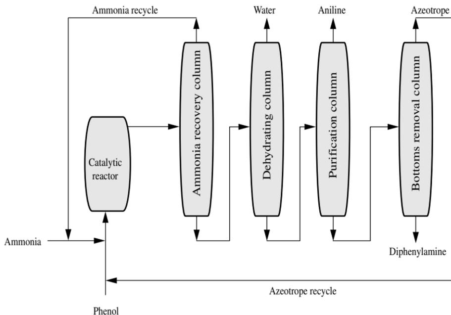
FIGURE 3 Aniline and diphenylamine production from phenol.
