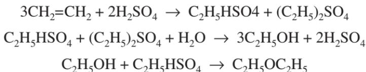
The conversion yield of ethylene to ethyl alcohol is 90 percent with a 5 to 10 percent yield of diethyl ether ( $\text{C}_2\text{H}_5\text{OC}_2\text{H}_5$ ).
