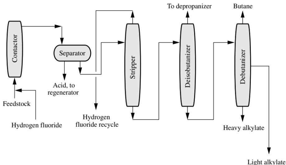
FIGURE 1 Alkylation using hydrogen fluoride.
