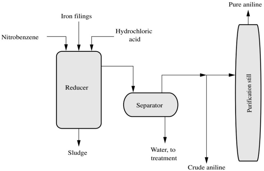
FIGURE 1 Aniline production by the reduction of nitrobenzene.
