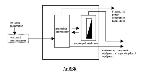
Figure 9.6 general process flow diagram of the AnMBR process
