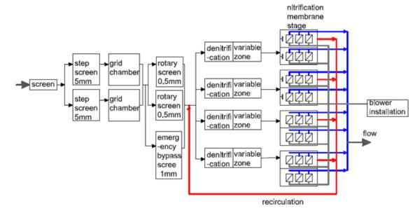
Figure 8.4 flow sheet of the Nordkanal waste water treatment plant
