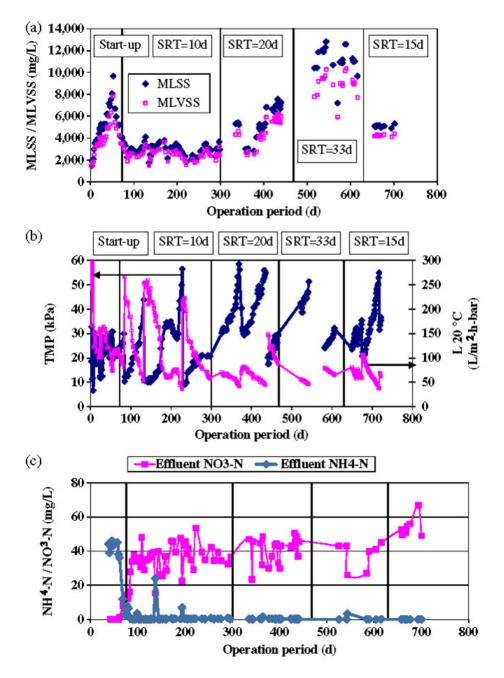
Figure 7.1 variation of (a) MLSS and MLVSS, (b) transmembrane pressure (TMP) and membrane permeability,(c) treated effluent  $NH_4$ -N and  $NO_3$ -N with time (Malamis et al. 2011).
