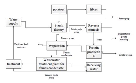
Figure 8.11 Flow chart of the treatment of process and potato pulp water at Emsland Starke GmbH
