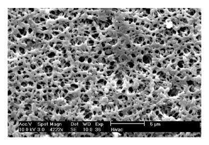
Figure 2.1 microscopy of morphology of membrane (Churchouse 2005).
