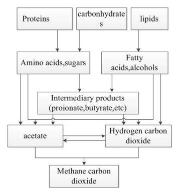
**Figure 9.2** Reactive scheme for the anaerobic digestion of polymeric materials. Numbers indicate the bacterial groups involved: 1. Hydrolytic and fermentative bacteria,
