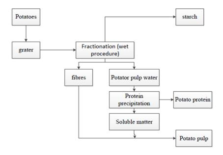
Figure 8.10 flow chart of potato starch production
