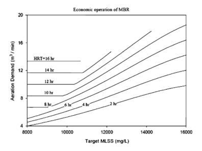
**Figure 5.1** aeration demands for biodegradation of organic matters as a function of target MLSS and HRT. Flow rate and COD of influent were 1000 m3/d and 400 mg/L, respectively (Radjenović et al. 2008).
