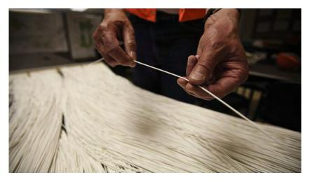
Figure 2.2 hollow fiber membranes
