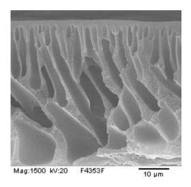
Figure 2.8 cross-section of a membrane
