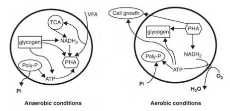
Figure 1.1 Metabolism of PAO under anaerobic and oxic conditions (van Haandel and van der Lubbe 2007)
