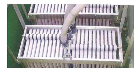
Figure 8.7 module cassettes during In-air cleaning
