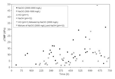
Figure 7.3 TMP decrease after chemical CIP with different cleaning reagents.
