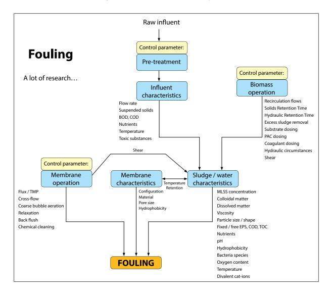
Figure 3.3 parameters influencing membrane fouling.
