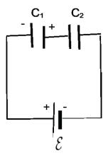
We consider two capacitors  $C_1$  and  $C_2$  connected in series, as shown. The charge on both capacitors are the same  $Q_1 = Q_2 = Q$ . We note that the voltage drops across the two capacitors add up to the electromotive force  $\mathcal{E} = V = V_1 + V_2$ . Since  $V_1 = Q/C_1$  and  $V_2 = Q/C_2$ , we write  $V = Q/C_{eq} = Q/C_1 + Q/C_2$ , or
