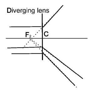
The incoming rays of an object (infinitely) far away are refracted in a *diverging* lens such that they diverge: their continuation backwards intersect at the focal point  $F_2$ : the distance between the center of the lens and the focal point is the focal length f. The focal point  $F_2$  is in front of the lens and we use the convention
