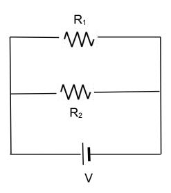
We consider two resistors  $R_1$  and  $R_2$  in parallel, as shown. The potential drops across the two resistors  $V_1$  and  $V_2$  is equal to the voltage of the battery:  $V = V_1 = V_2$ . Since  $I_1 = V/R_1$  and  $I_2 = V/R_2$  are the currents through the resistors  $R_1$  and  $R_2$ , respectively, the current through the battery is the sum  $I = I_1 + I_2$ . We introduce the equivalent resistance  $I = V/R_{eq}$  and find
