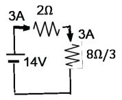
Thus the total resistance is  $R_{\rm tot}=2\,\Omega+8\,\Omega/3=14\,\Omega/3=4.67\,\Omega$
