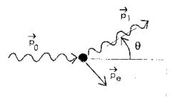
Electrons are elementary particles, i.e., they have no radius and also have no internal degrees of freedom. Thus, if a photon scatters off an electron [so-called Compton effect], the interaction can be analyzed by the condition of the conservation of energy:
