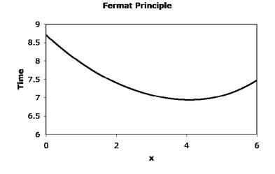
We assume that  $n_1 > n_2$  so that  $v_1 < v_2$ . In this case, the straight path from *A* to *B* does not correspond to the shortest time. Rather, as shorter time can be found by shortening the path from *A* to the interface and thus lengthening the path from the interface to *B*. That is, the condition of shortest time between *A* and *B* produces the bending of the path away from the normal, just as in the case of refraction.
