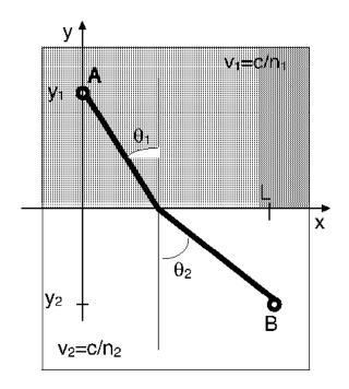
The phenomena of reflection and refraction can be explained by *Fermat's principle*; it states that the path taken by light in traveling from one point to another is such that the time of travel is a minimum. Fermat's principle can be used to qualitatively explain mirages and sunsets. Dispersion of light follows from the frequency dependence of the index of refraction n = n(f): violet is bent more than red [*rainbow!*].
