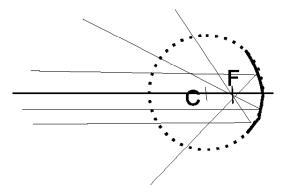
For a *concave* mirror, the reflected rays intersect at a point in front of the mirror; if a screen is placed at that location, a clear image of the object is seen on the screen [similar to a picture on the screen of a movie theater]. We say the image is *real*. If the object is (infinitely) far away the location of the image is at the *focal point* in front of the mirror. The distance between focal point and the mirror is the focal length:
