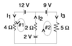
**Solution**: We have the three currents  $I_1$ ,  $I_2$ , and  $I_3$  as shown. We have for the two loops #1 and #2:
