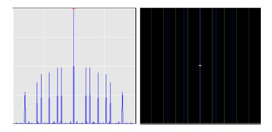
When the number N of slits is increased, the number of minima and maxima increases. The intensity of some minima does not change with N [principal maxima], whereas the intensity of great many maxima decreases as N increases [secondary maxima]. When N becomes of the order of hundred or thousand, the secondary minima can no longer be observed, and only the primary maxima 'survive.' This arrangement is called a diffraction grating. The angles of the m-th order principal maxima is given by
