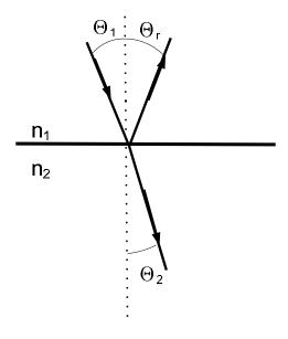
An interface exists between two media with different index of refraction  $n_1 < n_2$ . When incident ray at the angle  $\theta_1$  with respect to the normal strikes the interface, light is partially reflected at the angle  $\theta_r = \theta_1$  and partially refracted at the angle  $\theta_2 < \theta_1$ , i.e., the ray is refracted towards the normal. In the case  $n_1 > n_2$ , one finds  $\theta_2 > \theta_1$ , i.e., the ray is refracted away from the normal.
