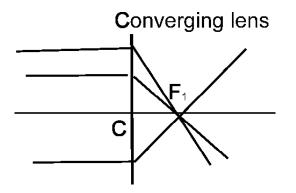
The incoming rays of an object (infinitely) far away are refracted in a *converging* lens such that they intersect at the focal point  $F_1$ : the distance between the center of the lens and the focal point is the focal length f. The focal point  $F_1$  is behind the lens and we use the convention
