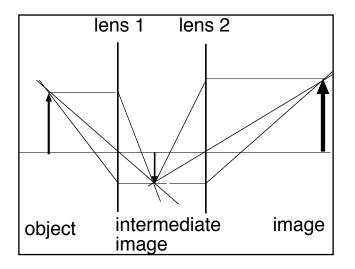
Both lenses are *converging*. The focal lengths are
