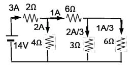
The same (1/3) A current through  $1\Omega$ ,  $2\Omega$  and  $3\Omega$  resistors:
