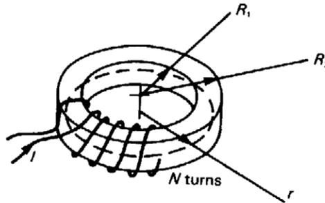
Fig 4.5. A coil wound on a ring-shaped former.
