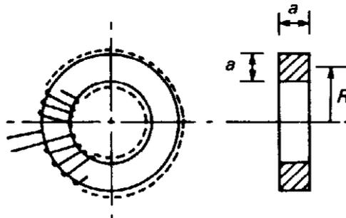
**Fig. 6.4.** The arrangement of a toroidal inductor.
