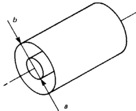
Fig. 1.7: The arrangement of an air-spaced coaxial line
