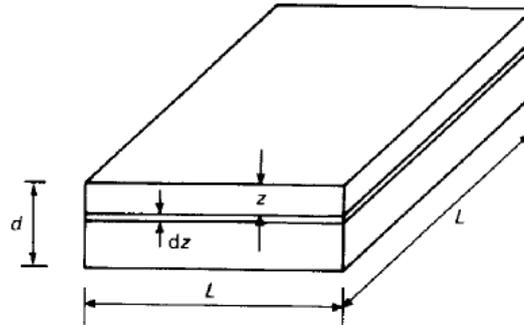
**Fig. 3.2** Calculation of the sheet resistance of an integrated-circuit diffused resistor.
