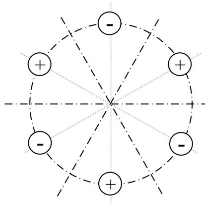
**Fig. 1.4** Image charges for planes intersecting at  $60^\circ$
