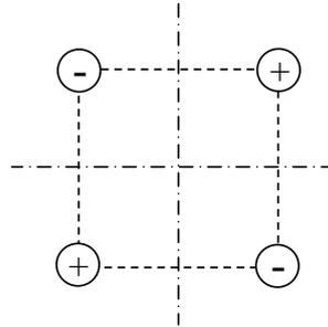
**Fig. 1.3** Image charges for planes intersecting at  $90^\circ$
