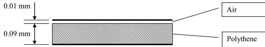
**Fig. 2.6** Capacitor with mixed dielectrics
