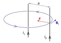
The force on a circuit in a magnetic field is given by Ampère's force law
