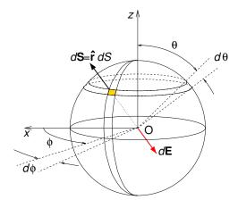
At the centre of the sphere the electric field due to the volume charge will be zero because the contribution of a volume element located at  $\mathbf{r}'$  will be exactly cancelled by that of an equivalent volume element at  $-\mathbf{r}'$ , so we only need to consider the surface charge.
