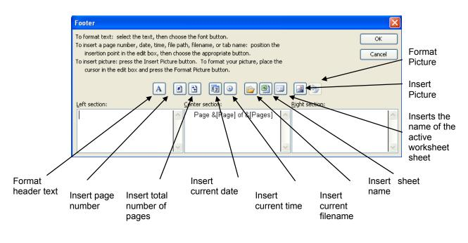
Figure 51 - Custom Header/Footer buttons
