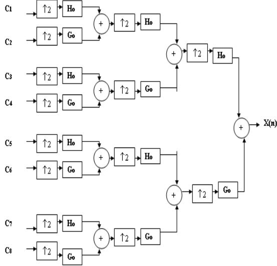
Figure 2: Three levels of wavelet Packet reconstruction tree.
