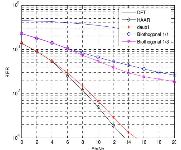
Figure 7: BER vs.  $E_b/N_0$  performance of MC-CDMA Based DWPT in the Rayleigh Fadding channel.
