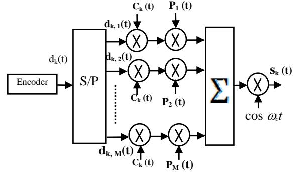
Figure 3: Transmitter Model.
