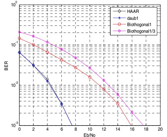
Figure 6: The BER vs.  $E_b/N_0$  performance of MC-CDMA BASED DWT in the AWGN channel.
