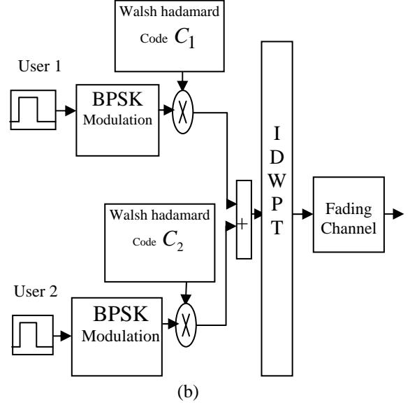
Figure 5: Simulated DWPT Based MC-CDMA Transceiver. [(a) Transmitter and (b) Receiver].
