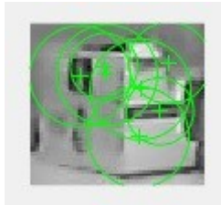
Figure 6: An example image of a reference object with 100 strongest feature points.
