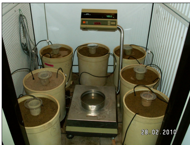
Figure 3. Ceramic pitchers buried in the soil pins inside controlled chambers.
