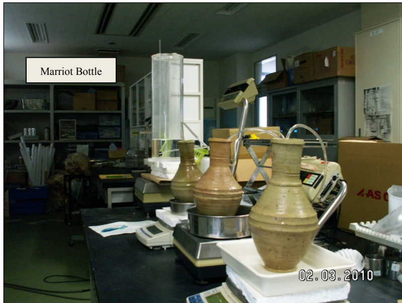
Figure 2. General view for the experimental setup. Measurement of seepage rate from the ceramic emitters (pitchers) in the atmosphere under constant head.
