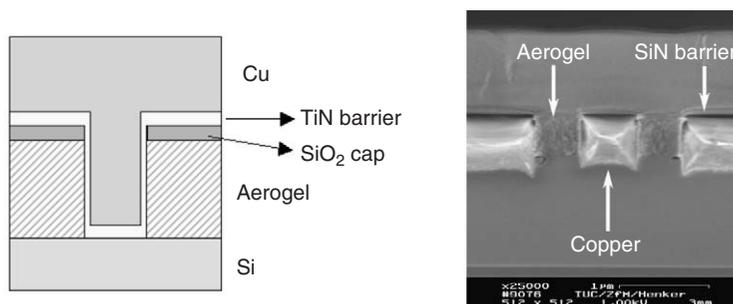
Fig. 8.38 Schematic of the structure before Cu CMP and cross-section SEM of polished single damascene structures in low- $k$  aerogel film.
