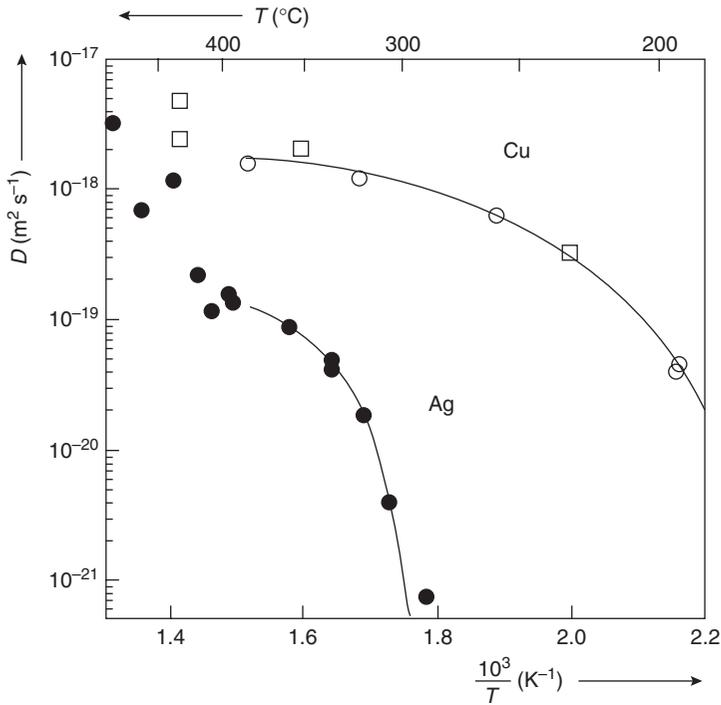
Fig. 6.11 Arrhenius plot for the diffusion of Cu and Ag atoms in polyimide. From Faupel [45].
