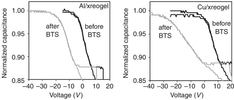
Fig. 9.36 CV curve for xerogel capacitors [177]: (a) Al-xerogel capacitors measured at a temperature of 100°C; (b) Cu-xerogel capacitors measured at temperature of 150°C (reprinted with permission).
