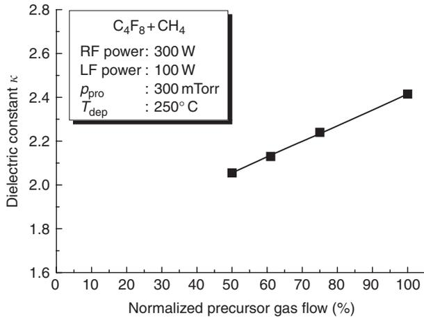
Fig. 7.11 Dielectric constant of CF polymer layers deposited from different  $C_4F_8/CH_4$  precursor gas flows.
