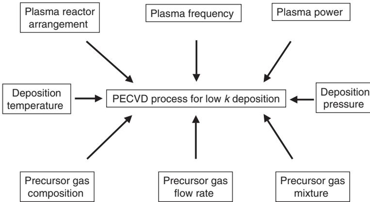
Fig. 7.5 Influence of process parameters on CF polymer deposition.
