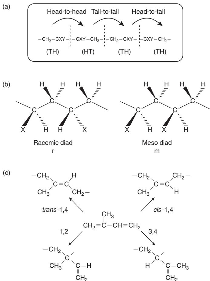
Fig. 6.2 (a) Shows head-to-head, tail-to-tail, and head-to-tail linkages in the same polymer, from the  $\text{CH}_2=\text{CXY}$  monomer. Same monomer may lead to all one type of linkages or a mixed one such as one shown here; (b) schematic diagram showing stereoisomerism in a diad (two  $\text{CH}_2=\text{CHX}$  monomer unit) polymer; and (c) four structural isomers of isoprene ( $\text{CH}_2=\text{C}(\text{CH}_3)-\text{CH}=\text{CH}_2$ ) [5] (reprinted with permission).
