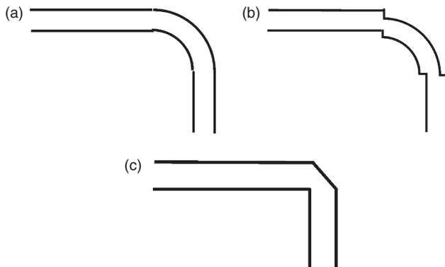
Fig. 11.4 (a) In-plane radius bend 90° turn; (b) Offset radius bend 90° turn; (c) Total internal reflection 90° bend using high-index materials.
