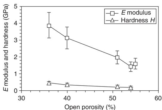
Fig. 8.29 Elastic modulus and hardness for porous SiO<sub>2</sub> aerogel films versus porosity measured by nano-indentation (adapted from [27]).
