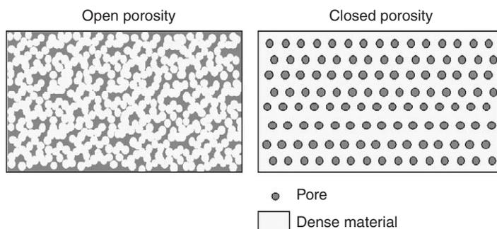
Fig. 8.24 Schematic of the open- and closed-pore structure in a porous material.
