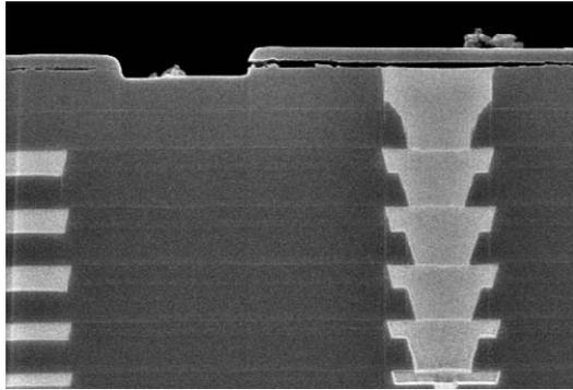
Fig. 4.10 SEM cross-sectional image of delamination at the interface of SiN and FSG at the terminal metal level.
