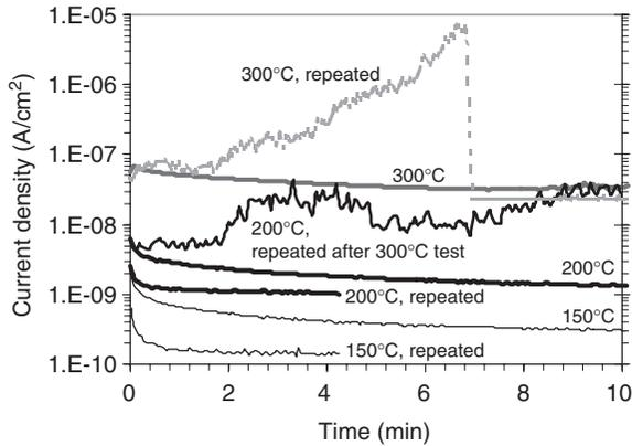
Fig. 9.34 Leakage currents for Cu on xerogel substrate [177] (reprinted with permission).
