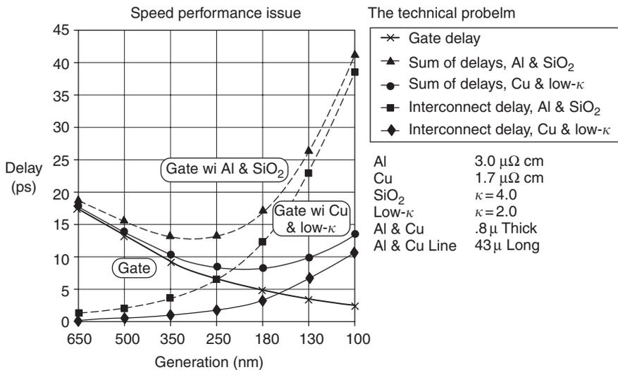
Fig. 9.2 Calculated gate and interconnect delay versus technology generation. (Adopted from the International Technology Roadmap for Semiconductors 1999).
