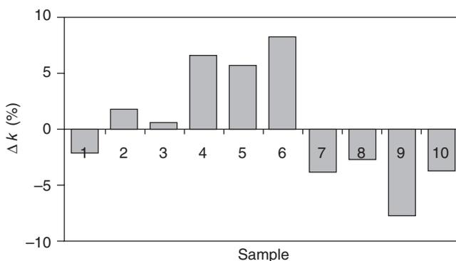
Fig. 8.33 Dielectric constant change after gas treatments or PECVD depositions on aerogel films [35].
