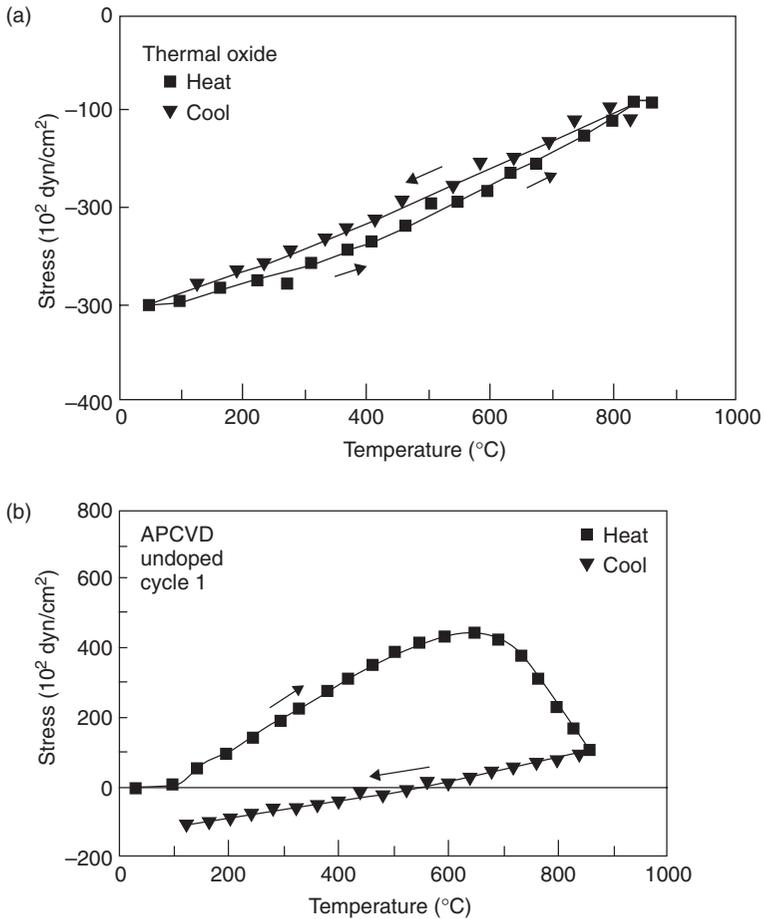
Fig. 2.5 Stress as a function temperature (*in situ* measurements) during heating/cooling cycles of (a) thermally grown SiO<sub>2</sub> films and (b) APCVD SiO<sub>2</sub> films (from Ref. [30]).
