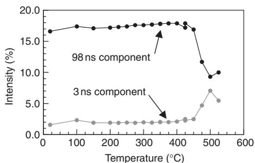
Fig. 3.12 Ps lifetime intensity as a function of annealing temperature after 1 h. for positrons implanted into a Nanoglass film capped with sputtered aluminum. The 98 ns component is characteristic of the 7.7 nm pores that were measured in TEOS-capped Nanoglass films. The 3 ns component is characteristic of pores coated and closed off by diffused aluminum.
