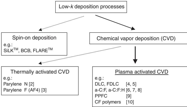
Fig. 7.1 Low-*k* deposition processes for carbon-based materials.
