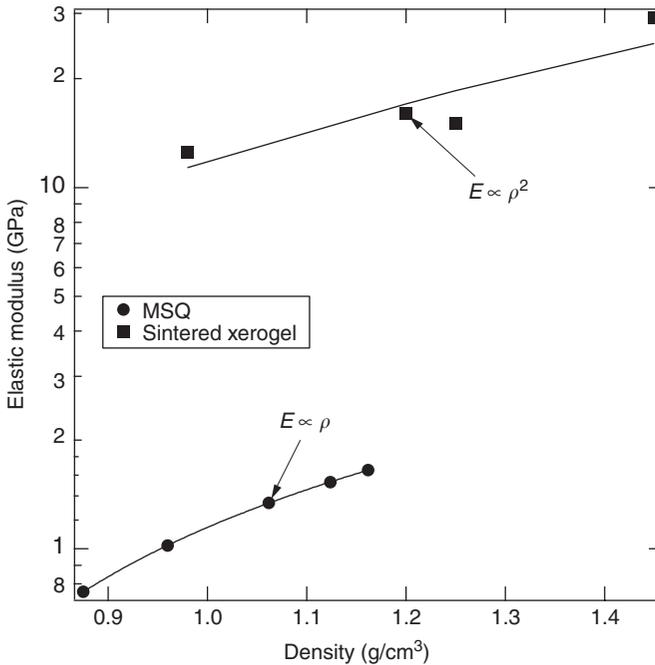
Fig. 9.26 Elastic modulus of MSQ and sintered xerogel materials as a function of density. Data measured using surface acoustic wave (MSQ) [79] and nanoindentation (xerogel) [61] techniques.
