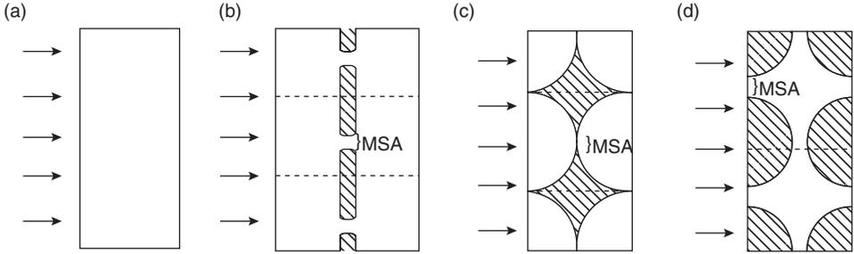
Fig. 9.13 Concept of minimum solid area. (a) shows a uniform body on which uniform stress is impinging. (b) Shows a body with isolated pores (hatched), MSA is the major factor controlling the transmittal of stress. (c) and (d) show, respectively, the idealized bodies, respectively, of bonded uniform spherical particles or an idealized foam [81] (reprinted with permission).
