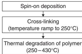
Fig. 8.10 Example for process flow for controlled templated polymerisation of MSQ/PCL two-phase system to produce porous silica.
