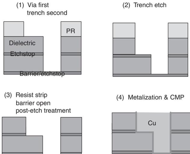
Fig. 5.26 Dual damascene scheme for copper processing.
