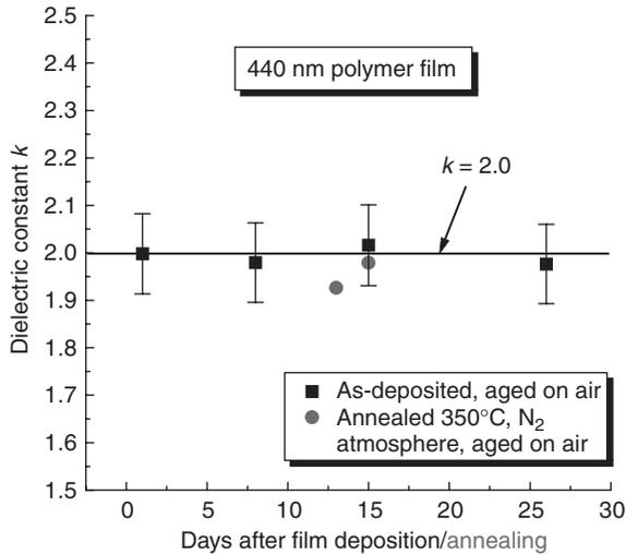
Fig. 7.20 Aging of CF polymer layer [10].
