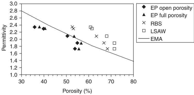
Fig. 8.25 Dielectric constant (permittivity) measured by different techniques for aerogel films of varying porosity.
