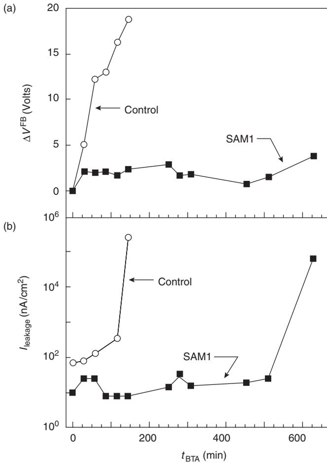
Fig. 6.15 (a) Flatband voltage shift,  $\Delta V^{FB}$  and (b) leakage current density, leakage, plotted as a function of  $t_{BTA}$  for control and SAM1 capacitors. From Krishamoorthy *et al.* [138].
