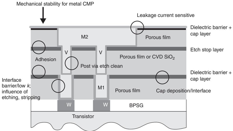
Fig. 8.31 Schematic of a dual damascene copper metallisation scheme using porous low- $k$  dielectric.
