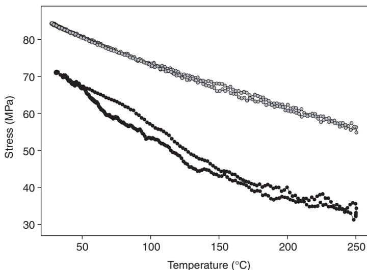
Fig. 3.14 Thermal stress measurements for two different OSGs on Si. The lower curve is more noisy because it was obtained from a film on a 700  $\mu\text{m}$  thick substrate, after extending the light path to 6 m.
