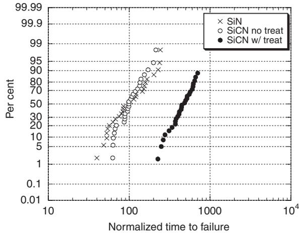
Fig. 4.16 Electromigration performance of SiCN as a function of pre-treatment used.
