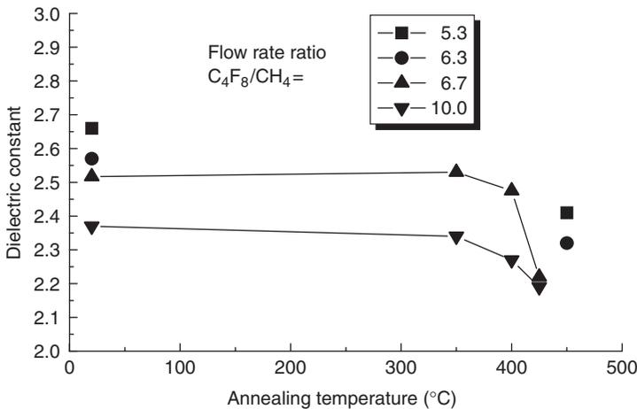
Fig. 7.12 Influence of annealing temperature and  $C_4F_8/CH_4$  flow rate ratio on the dielectric constant of CF polymers [10].
