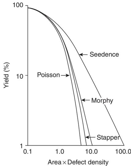
Fig. 12.1 A comparison of the yield obtained using different defect distribution functions (see Table 12.2). From Parks [19].
