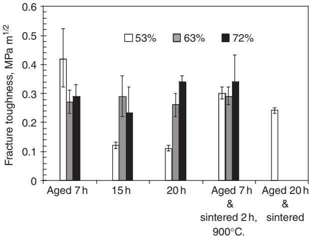
Fig. 9.20 Fracture toughness for xerogel films as a function of process history [61] (reprinted with permission).
