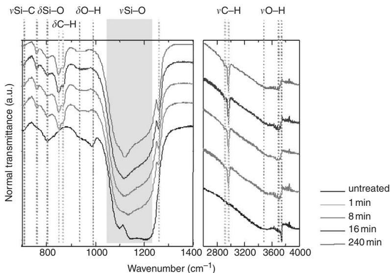
Fig. 8.20 FTIR spectra for HMDS treatment of aerogels for varying exposure times [19].
