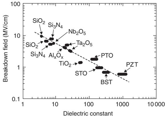
Fig. 2.2 A log–log plot of the dielectric breakdown field (for  $10^{-6}$  A current) as a function of the dielectric constant of the dielectric (from Ref. [17]).
