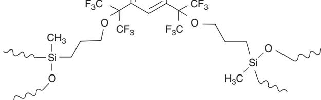
Fig. 6.8 Representative structure of: (a) fluorinated polyimide copolymers; (b) fluoro aromatic triallyl-ether copolymer.
