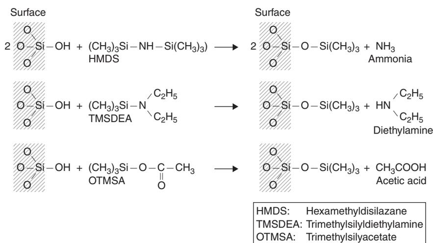
Fig. 8.19 Scheme of the balance reactions for the different hydrophobisation chemicals (after [19]).
