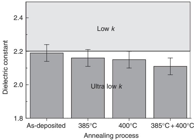
Fig. 7.13 Dielectric constant of CF polymer after annealing in vacuum [29] (© 2001 IEEE).
