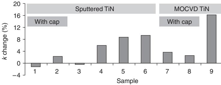
Fig. 8.37 Relative change of dielectric constant  $k$  after diffusion barrier deposition using different processes on capped and non-capped aerogel compared to the untreated state [35].
