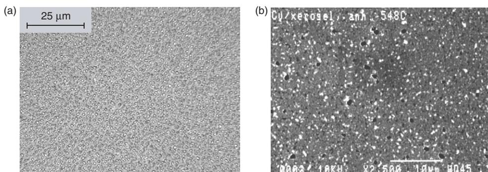
Fig. 9.27 Micrographs showing the morphology of Cu on solid  $\text{SiO}_2$  and on xerogel upon annealing: (a) Cu on  $\text{SiO}_2$  annealed at  $450^\circ\text{C}$  in  $\text{N}_2$ ; (b) Cu on 70% porous xerogel annealed at  $548^\circ\text{C}$  in  $\text{N}_2$  [177] (reprinted with permission).
