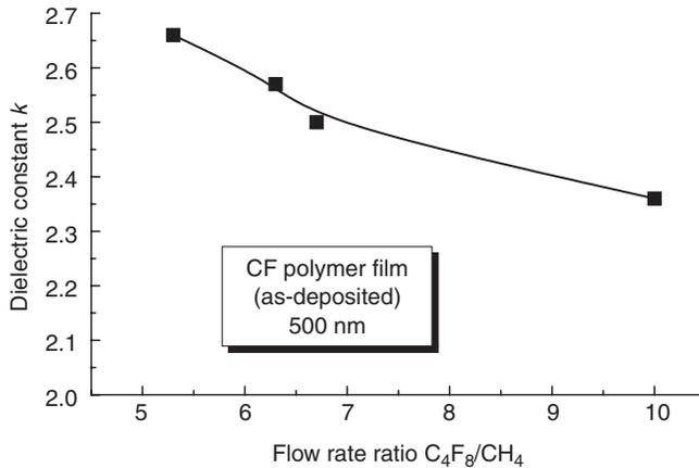
Fig. 7.10 Dielectric constant of CF polymer layers deposited from different  $C_4F_8/CH_4$  precursor gas mixtures.
