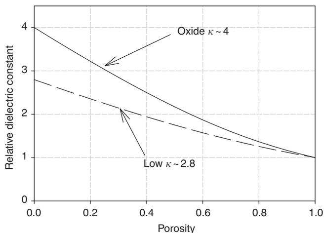
Fig. 3.1 Bruggeman's EMA showing dielectric constant vs. porosity for oxide and a low- $\kappa$  material.
