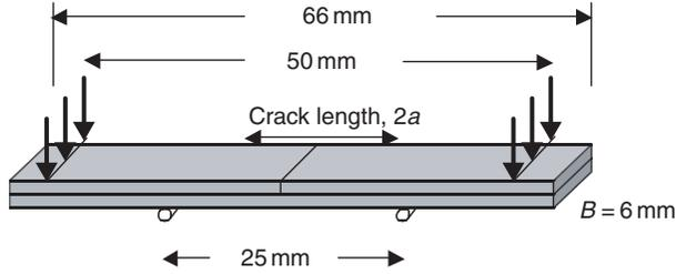
Fig. 3.2 Typical sample configuration for four-point bend test.
