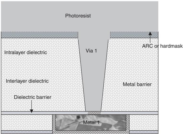
Fig. 4.3 Drawing of etched via prior to trench patterning for a VFTL integration.
