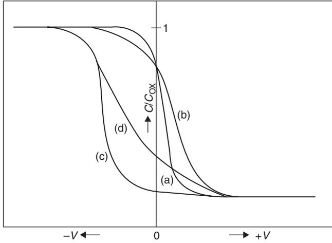
Fig. 2.3 Typical  $C$ - $V$  curves for ideal (a) and non-ideal behaviors (b), (c), and for a MOS or MIS capacitor on p-type semiconductor (d).
