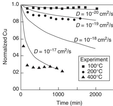
Fig. 9.31 Cu ion concentrations in a Flare™ low- $\kappa$  dielectric film upon heating at 200°C for 12 h. Notice the great change in diffusivity when the heated polymer passed its glass transition temperature (redrawn from data presented in [189] with permission).
