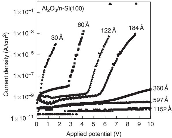
Fig. 10.4 Current–voltage ( $IV$ ) plots for  $\text{Al}_2\text{O}_3$  ALD films of different thicknesses grown on n-Si(100) at  $177^\circ\text{C}$ .
