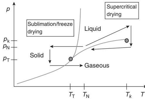
Fig. 8.5 Phase diagram showing two gel drying approaches for avoiding the liquid–gaseous transition.
