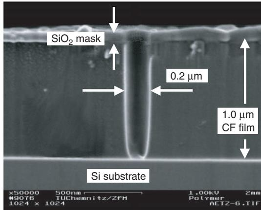
Fig. 7.19 ICP etched via22 (O<sub>2</sub> plasma) [10].
