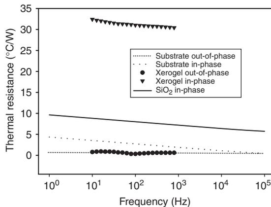
Fig. 3.7 Experimental  $3\omega$  data for in-phase and out-of-phase thermal resistance of a  $0.60 \mu\text{m}$  thick 48% porous xerogel film. The calculated thermal resistance for the substrate and a  $\text{SiO}_2$  film are also shown for comparison. Note that the thermal resistance is calculated from the in-phase component.
