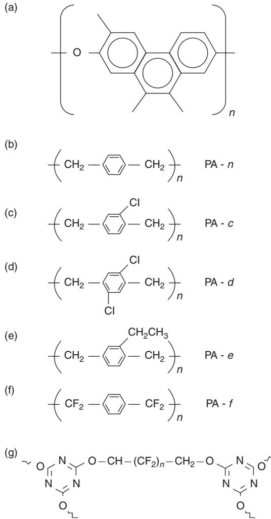
Fig. 6.7 Representative structures of: (a) SILK; (b-f) five different parylenes; (g) fluoromethylene cyanate ester.
