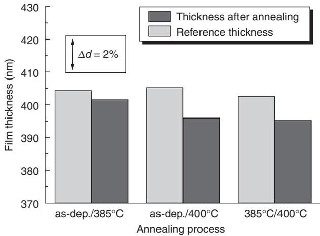
Fig. 7.9 Thickness change of CF polymer films annealed 30 min at highest temperature in vacuum [29] (© 2001 IEEE).
