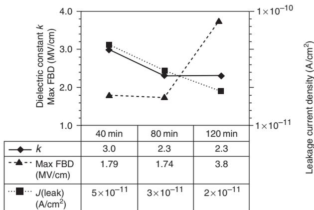
Fig. 8.17 Electrical parameters of aerogel films for different spin-on times after catalyst addition.
