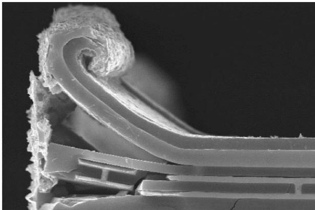
Fig. 4.9 SEM cross-sectional image of the scribed edge of a die.
