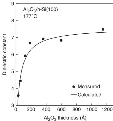
Fig. 10.5 Comparison of the measured and calculated dielectric constants for  $\text{Al}_2\text{O}_3$  ALD films of different thicknesses grown on n-Si(100) at  $177^\circ\text{C}$ .
