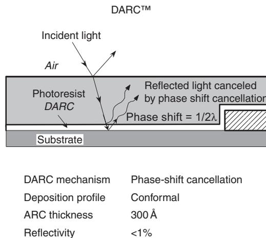
Fig. 5.33 Dielectric ARC works by phase-shift cancellation.
