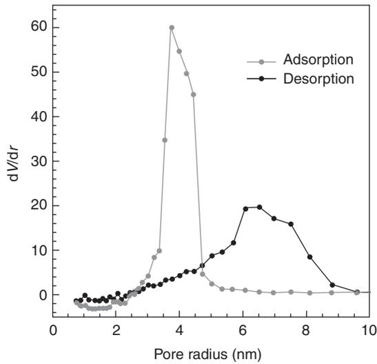
Fig. 8.26 Pore size distribution for porous SiO<sub>2</sub> with 55% porosity measured by EP.
