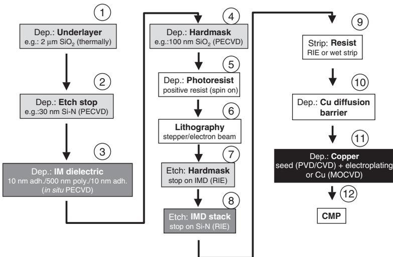
Fig. 7.17 Damascene process flow adopted to special requirements for CF polymer IMD.
