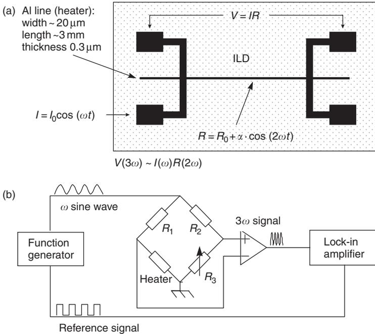
Fig. 3.6 (a) Top view of  $3\omega$  sample showing the metal line structure; (b) Experimental configuration for  $3\omega$  measurement. The sample (heater) is incorporated into a Wheatstone bridge to eliminate noise, while the signal is isolated using a lock-in amplifier.
