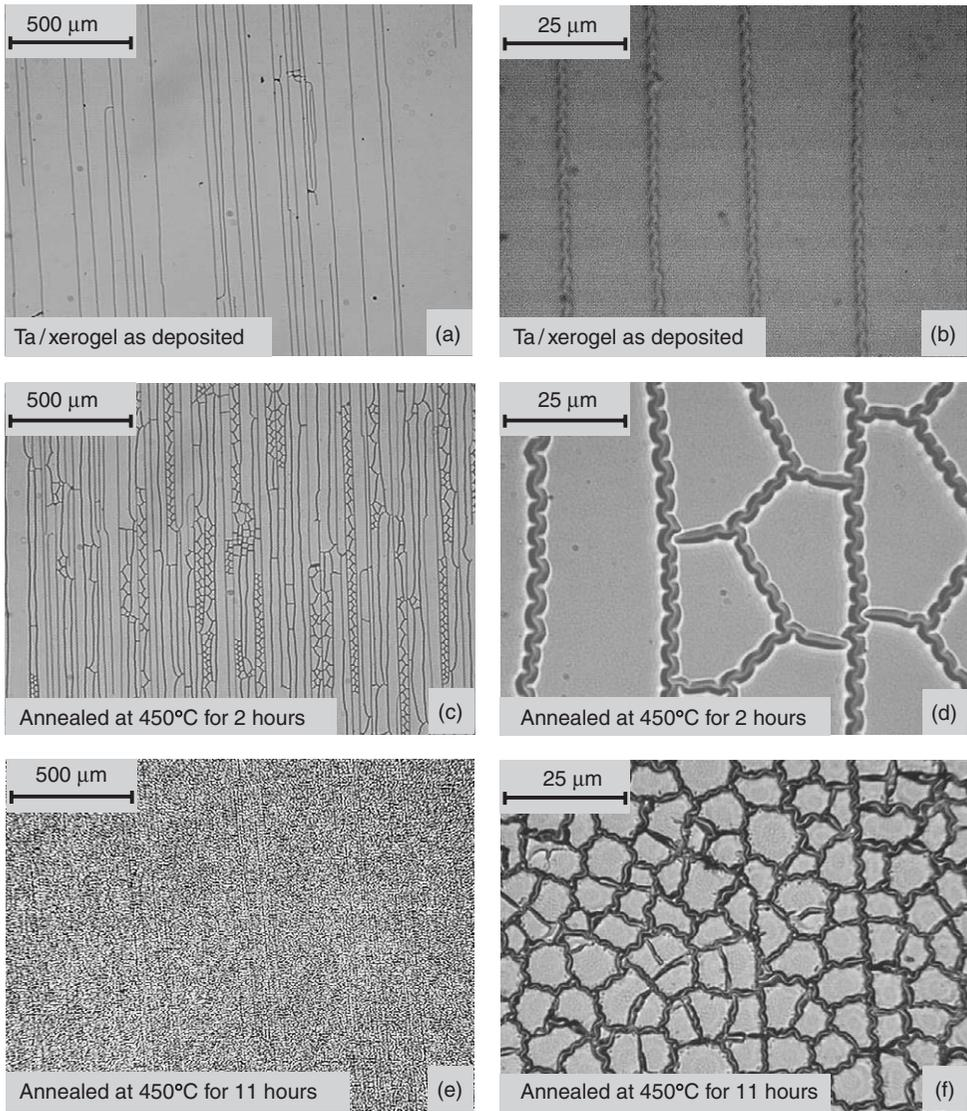
Fig. 9.28 Ta instability on xerogel surface [184] showing the classic telephone cord morphology.
