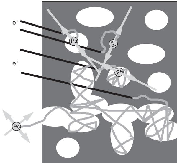
Fig. 3.11 An illustration of (PALS). The vacuum Ps lifetime (~142 ns) is shortened in the voids due to collisions with the void walls that increase the probability of annihilation into gamma rays. The Ps lifetime is measured by monitoring the gamma rays, and the lifetime is related to the average pore size.
