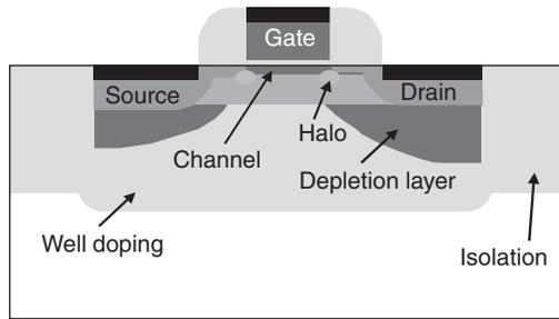
Fig. 13.4 Planar CMOS structure.
