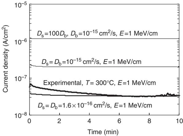
Fig. 9.39 Anode currents as a function of increasing surface diffusivity [177, 205] ( $Pe = 2000$ ) (reprinted with permission).
