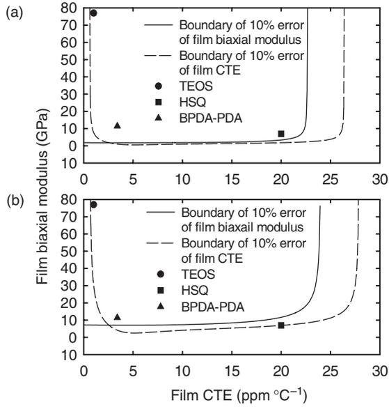
Fig. 3.4 Applicable regions of dual substrate bending beam method for 1  $\mu\text{m}$  thick films: (a) 125  $\mu\text{m}$  thick Si and Ge; (b) 250  $\mu\text{m}$  thick Si and 300  $\mu\text{m}$  thick GaAs. Plot assumes 0.5% error in film, substrate thickness and substrate modulus and a CTE, curvature error of  $2.1 \times 10^{-4} \text{ m}^{-1}$ .
