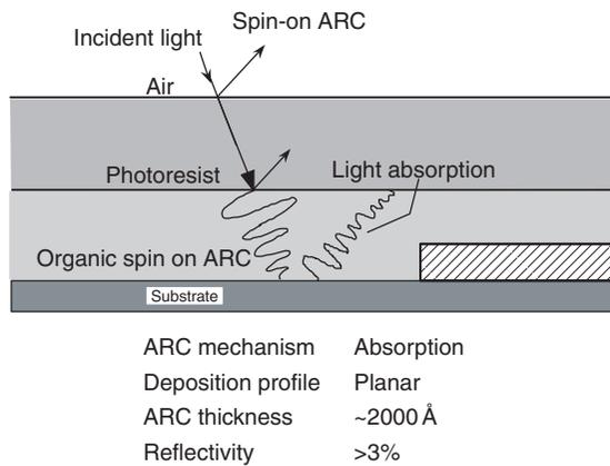
Fig. 5.32 Organic spin-on ARC works by absorption.
