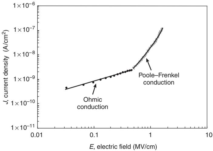
Fig. 9.9  $J$  versus  $E$  characteristics of a 60% xerogel film. The leakage current shows Ohmic conduction behavior at low fields [61] (reprinted with permission).
