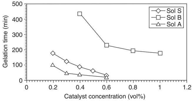
Fig. 8.14 Gelation time versus HF catalyst concentration for low-*k* aerogel.
