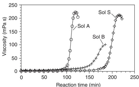
Fig. 8.4 Viscosity evolution over time during sol-gel processing for different sols (composition see Section 8.2.2.2).
