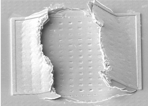
Fig. 4.15 Delamination along FSG/barrier interface upon wirebonding, when FSG is used as final ILD.
