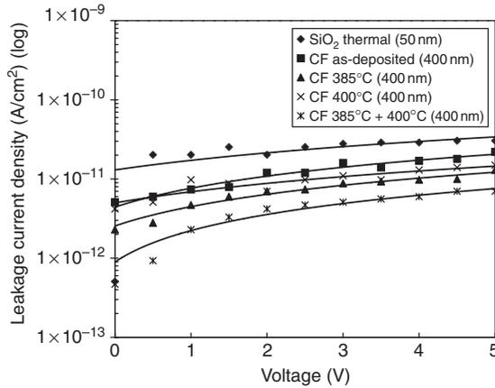
Fig. 7.14 Leakage current density of 400 nm CF polymer films (as-deposited and annealed up to 400°C) in comparison to SiO<sub>2</sub>.
