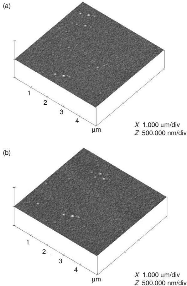
Fig. 7.8 (a) AFM plot of CF polymer (as-deposited). (b) AFM plot of CF polymer surface (annealed at 400°C in vacuum) [29] (© 2001 IEEE).
