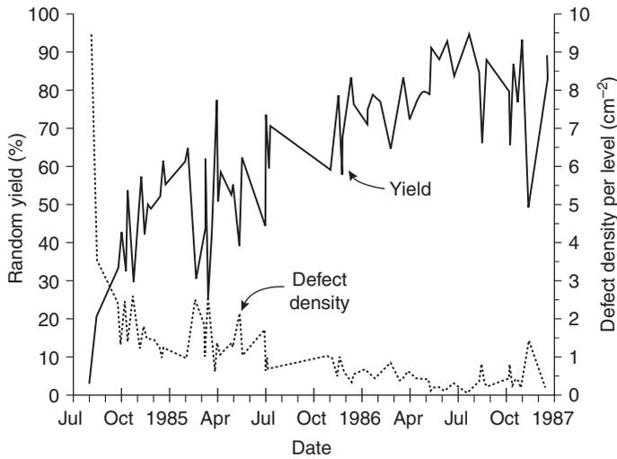
Fig. 12.2 Experimentally determined yield-defect relationships in a fabrication line. From Parks [19].
