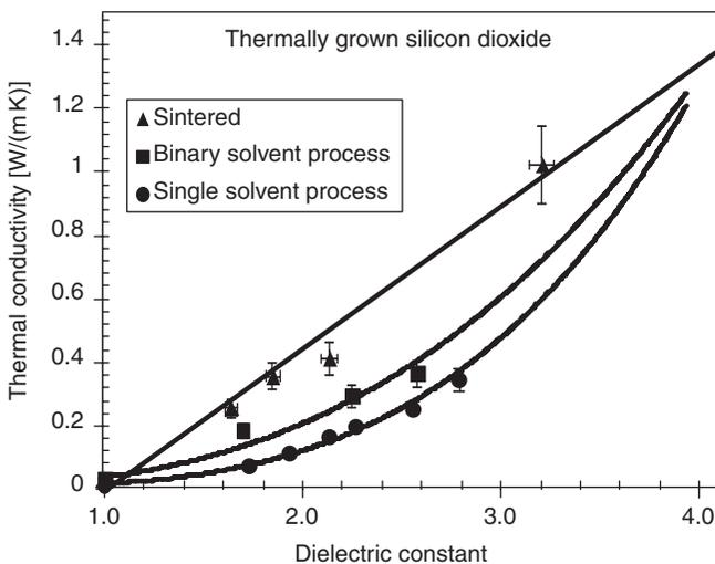
Fig. 9.23 Silica xerogel thermal conductivity as a function of dielectric constant [21] (reprinted with permission).
