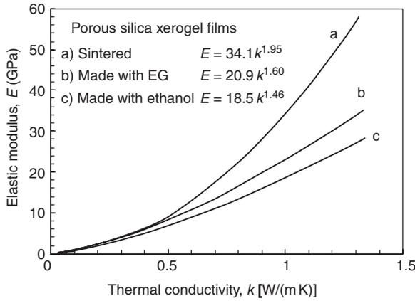
Fig. 9.25 Relationship between the thermal conductivity and elastic modulus for xerogel materials as a function of their processing history [21] (reprinted with permission).
