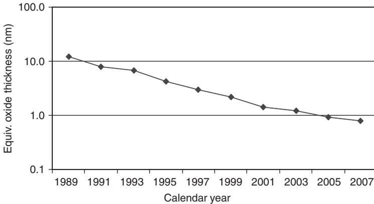
Fig. 13.3 Gate dielectric thickness scaling with time.
