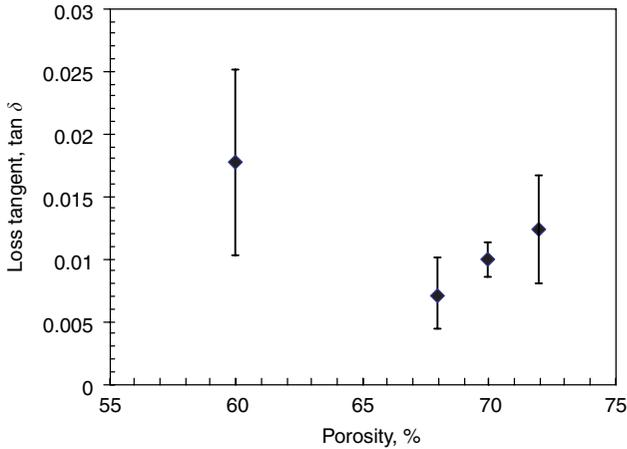
Fig. 9.8 Loss tangent measurements at 1 MHz for xerogel films of different porosity measured under ambient conditions [61] (reprinted with permission).
