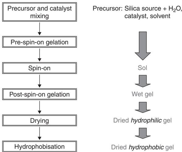
Fig. 8.6 Example of a general process flow to produce aerogel/xerogel films by solvent evaporation drying.
