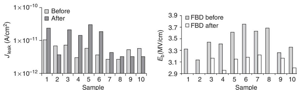
Fig. 8.34 Leakage current density (left) and field breakdown after gas treatments or PECVD depositions on aerogel films adapted from [35].
