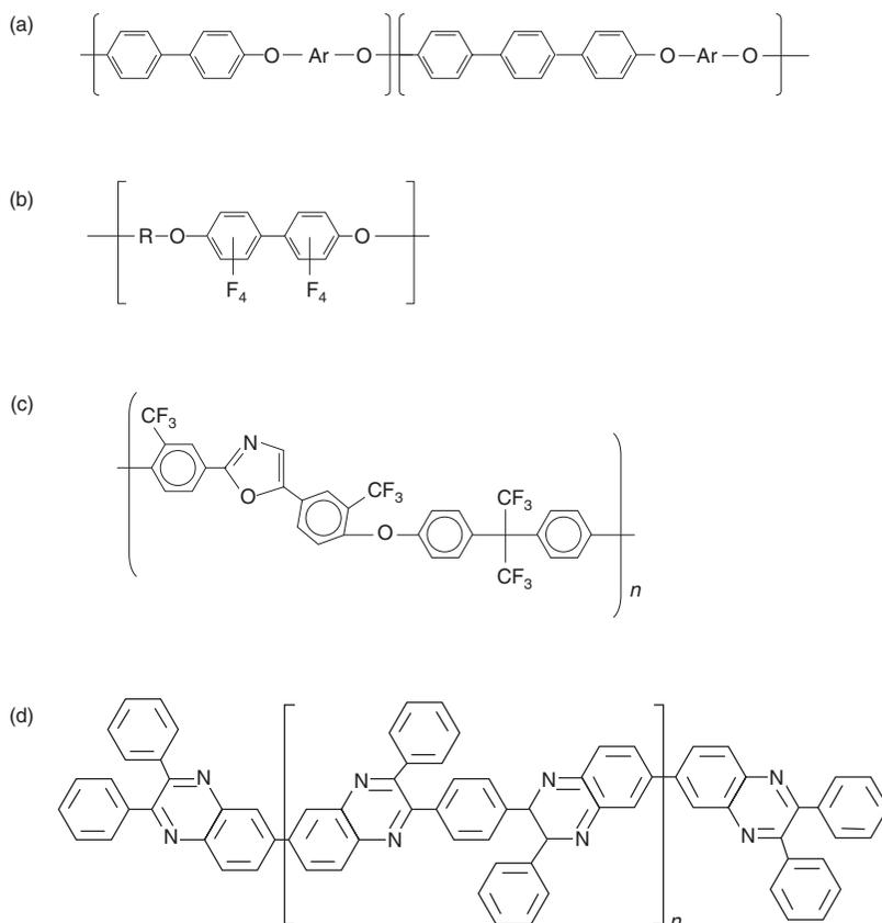
Fig. 6.5 Representative structures of: (a) poly(arylethers); (b) fluorinated poly(arylethers) (one of them is FLARE™); (c) poly(arylene ether oxazole); (d) polyphenylquinoxaline.
