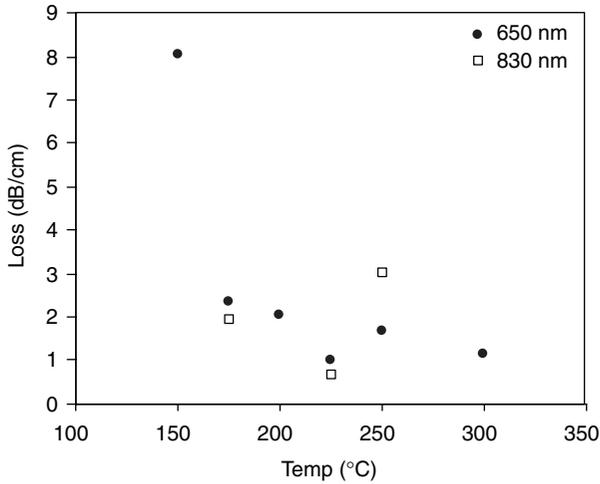
Fig. 9.10 Losses for oxide-40% porous xerogel planar waveguides at 650 and 830 nm [60] (reprinted with permission).
