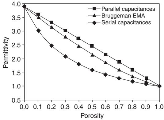
Fig. 8.2 Permittivity of porous SiO<sub>2</sub> versus porosity.
