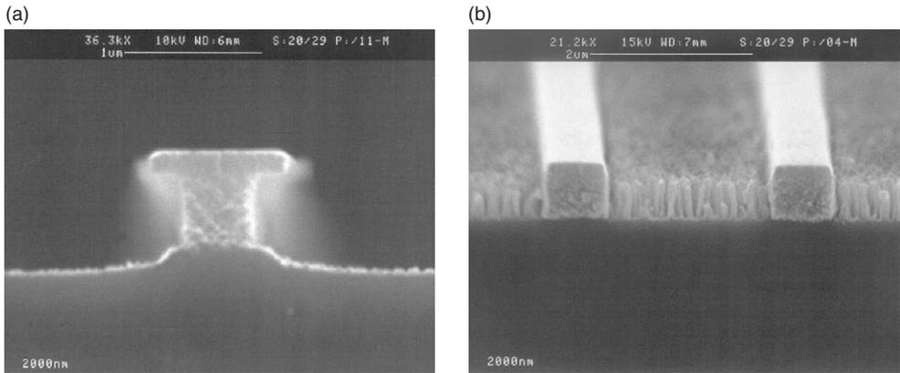
Fig. 8.35 Standard SiO<sub>2</sub> etching: (a) with ICP (b) without ICP.
