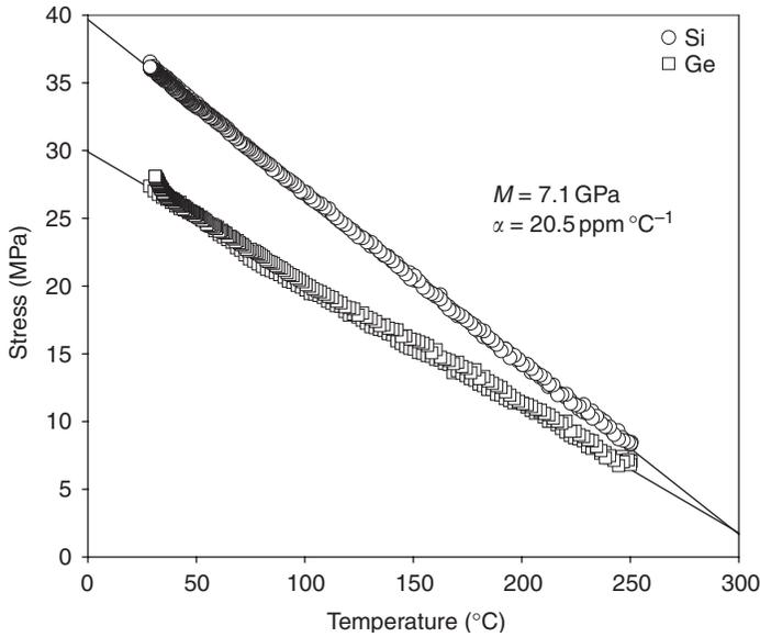
Fig. 3.5 Thermal stress data from dual-substrate bending beam measurement of 0.5 mm thick HSQ films on Ge and Si substrates. The biaxial modulus and CTE were determined to be 7.1 GPa and 20.5 ppm  $^{\circ}\text{C}^{-1}$ , respectively.
