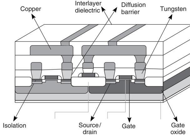
Fig. 9.1 A simplified cross-section of an IC showing the transistor (made up of source, gate, and drain) and the various levels of interconnect [61].
