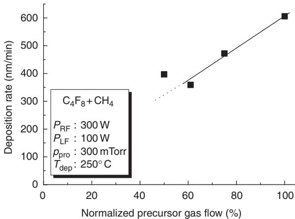
Fig. 7.6 Film deposition rate of CF polymers deposited at different normalized precursor gas flows.
