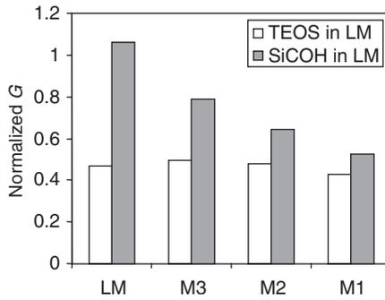
Fig. 4.12 Modeling results of the influence of final ILD on crack driving force at lower levels comparing TEOS and SiCOH as final ILD.
