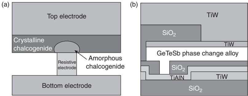
Fig. 13.11 Ovonic unified memory cell technology: (a) OUM cell technology; (b) Cross-section of cell structure. (Source: Ref. [19] and www.ovonyx.com).
