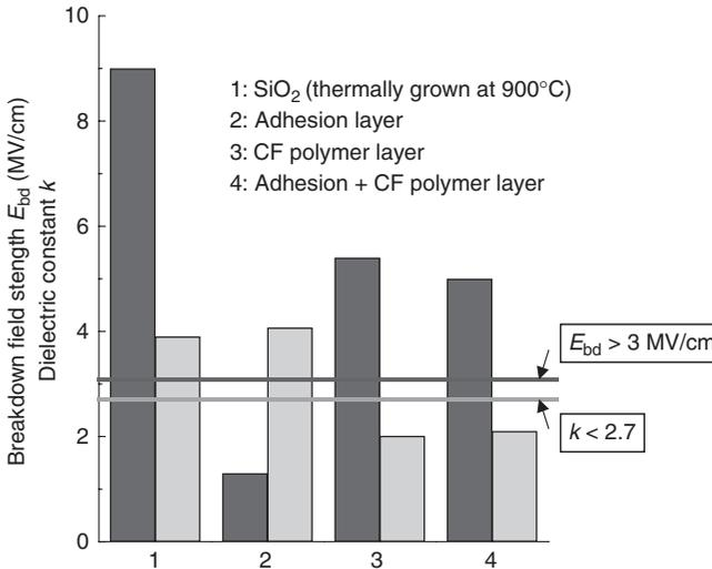
Fig. 7.15 Electrical properties of polymer layer stack in comparison to SiO<sub>2</sub> dielectric [29] (© 2001 IEEE).
