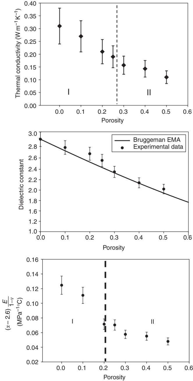
Fig. 3.16 Porosity dependence of material properties of porous MSQ films: (a) dielectric constant (curve shows the Bruggeman EMA); (b) thermal conductivity; and (c) thermal stress. In (c), the slope of thermal stress vs. temperature is shown, where  $2.6 \text{ ppm } ^\circ\text{C}^{-1}$  is the CTE of the silicon substrate and  $E(1 - \nu)^{-1}$  is the biaxial modulus. The transition from region I to region II due to percolation is clearly observed.
