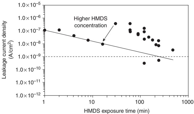
Fig. 8.22 Aerogel leakage current density versus HMDS exposure time.
