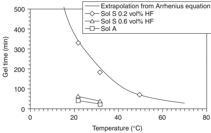
Fig. 8.15 Gelation time versus temperature for different sols.
