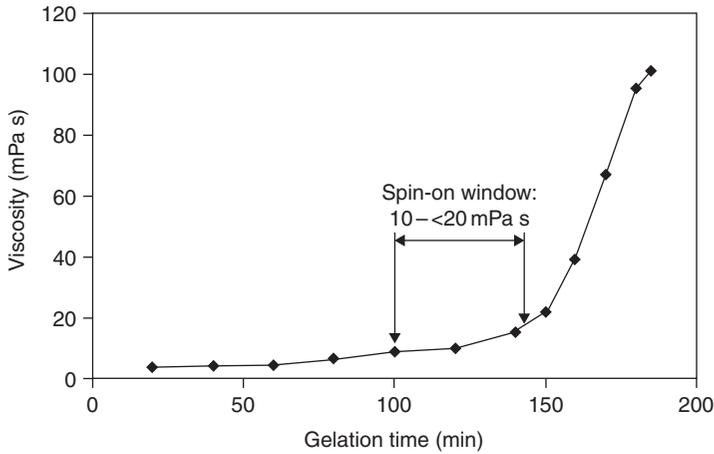
Fig. 8.11 Process window for spin on during gelation period.
