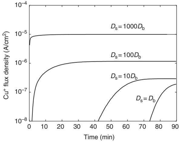
Fig. 9.41 Cu<sup>+</sup> current flux at the cathode ( $x = L$ ) showing breakthrough behavior ( $Pe = 2000$ ) [177, 195] (reprinted with permission).
