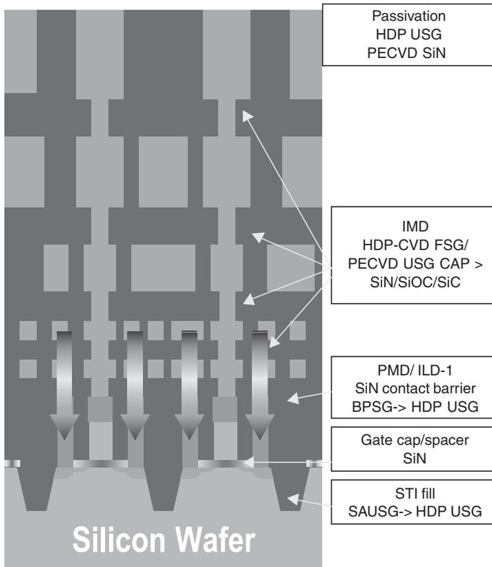
Fig. 5.17 Silicon-based dielectric layers in logic devices.
