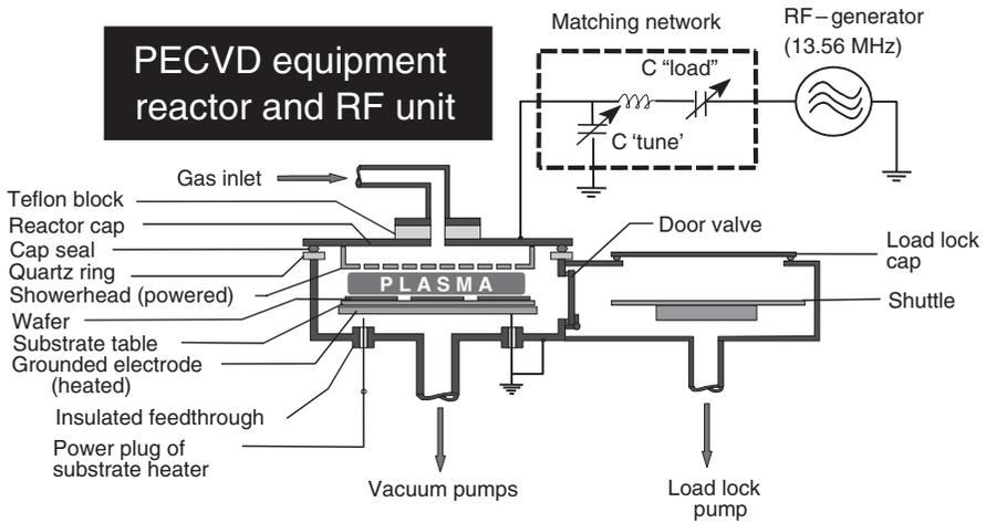
Fig. 7.2 Schematic of a PECVD deposition tool.
