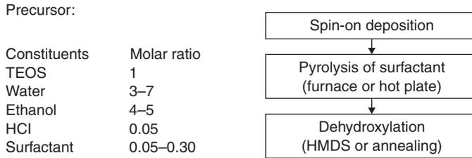
Fig. 8.9 Example of precursor composition and process flow for surfactant-templated silica.
