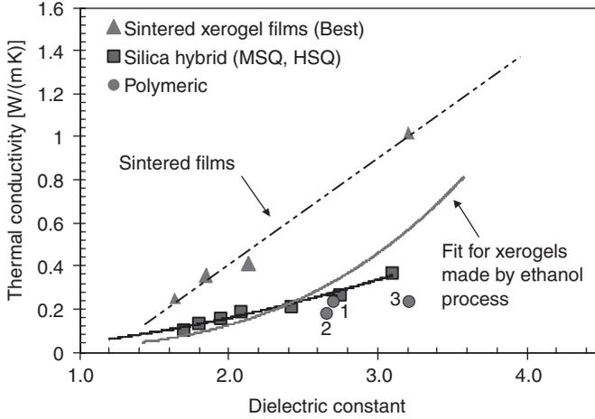
Fig. 9.24 A comparison of the thermal conductivity for low-κ materials [21] (reprinted with permission).
