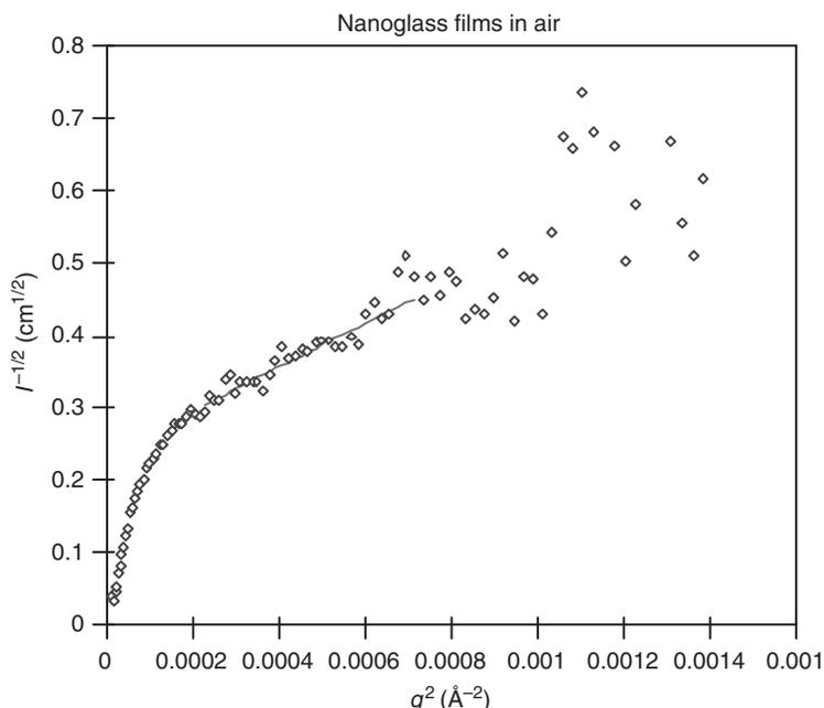
Fig. 3.10 Debye plot derived from an SANS experiment on a stack of Nanoglass thin films coated on silicon substrates. The slope of the fitted line provides the correlation length of the porous structure from which the chord length (average pore size) is calculated. The intercept of the fitted line at  $q^2 = 0$  gives a measure of the porosity and the mass density of the connecting material between the pores (pore wall material).
