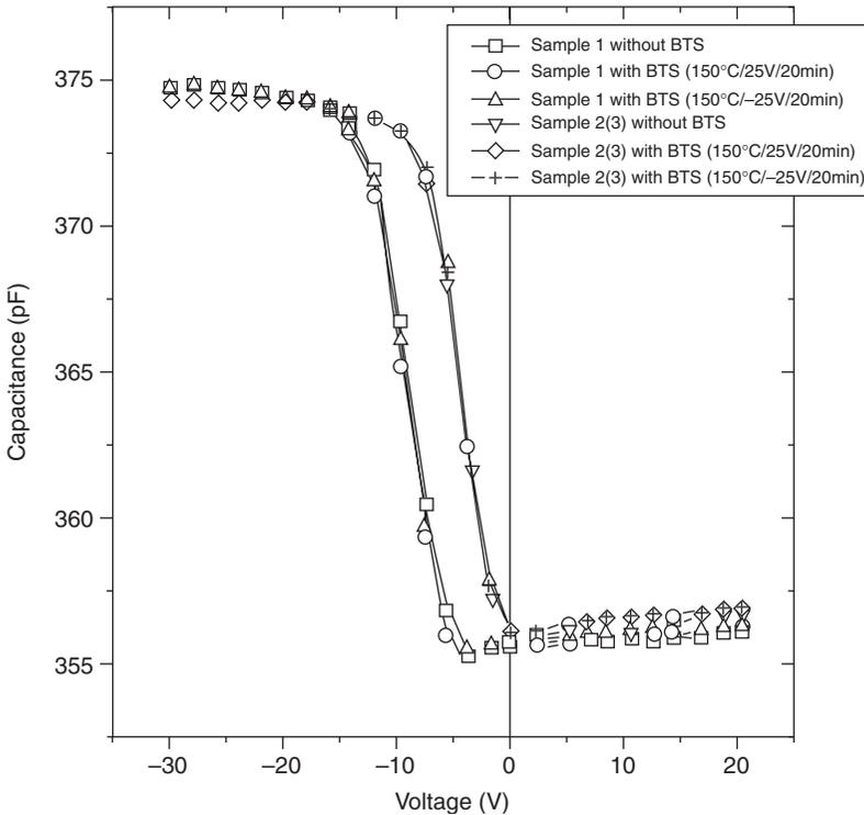
Fig. 6.12 High frequency (1 MHz)  $C-V$  characteristics of samples 1, 2, and 3 annealed, respectively, at 325, 350, and 375°C and then tested with or without BTS. From Lee [53].
