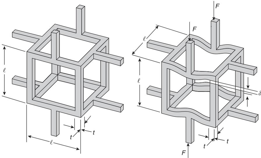
Fig. 9.11 Unit cell for an open-cell foam of cubic symmetry [80] (reprinted with permission).
