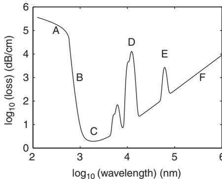
Fig. 11.6 Schematic summary of absorption processes in semiconducting solid materials. Letters label general classifications of transition: (A) electronic band-to-band transition; (B) exponential band tail; (C) electronic defect absorption; (D) vibrational transitions; (E) impurity absorption; (F) free carrier absorption.
