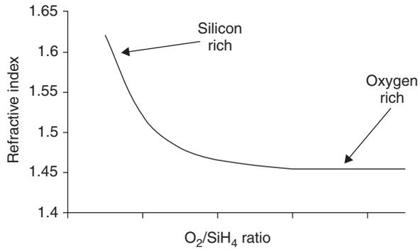
Fig. 5.7 Refractive index as a function of O<sub>2</sub>/SiH<sub>4</sub> ratio.
