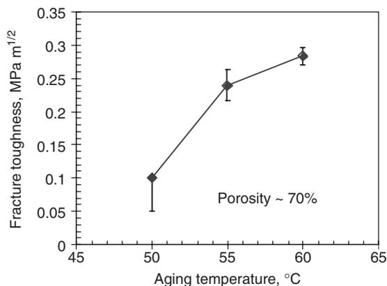
Fig. 9.19 Fracture toughness of xerogel films as a function of aging temperature [61] (reprinted with permission).
