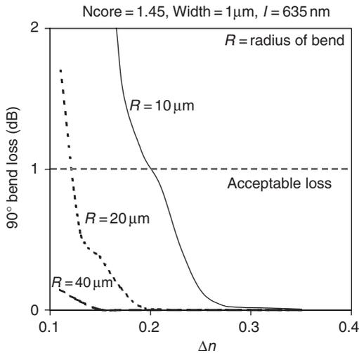
Fig. 11.12 Radiation loss plotted as a function of core-cladding index difference for 635 nm light passing through a  $90^\circ$  radius bend for various radii. The cladding index is 1.46 and the waveguide dimensions are  $1000 \text{ nm} \times 1000 \text{ nm}$  (from Ponoth [49]).
