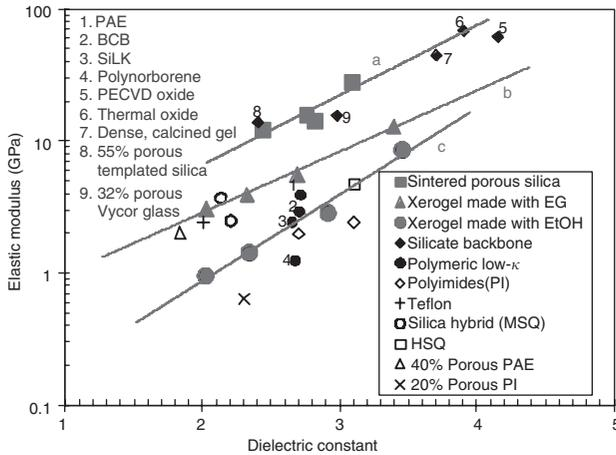
Fig. 9.17 Elastic modulus of various low- $\kappa$  materials. Solid lines are exponential best fits for xerogel films made with (curve b) and without ethylene glycol (curve c) and sintered films (curve a) [22] (reprinted with permission).
