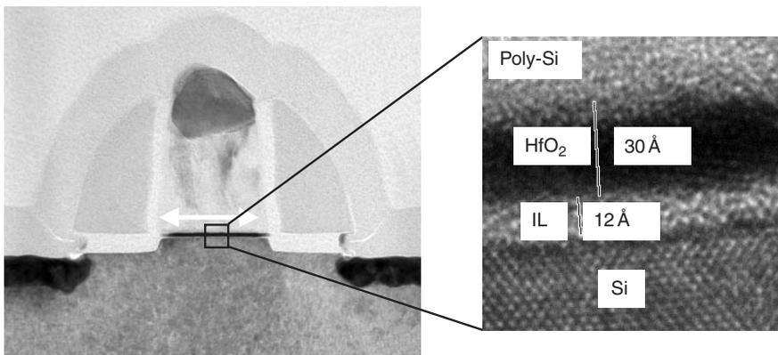
Fig. 4.6 Cross-sectional TEM of gatestack with  $\text{HfO}_2$  gate dielectric showing significant interfacial layer resulting from post-deposition anneal.
