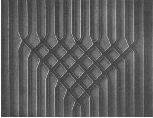
Fig. 11.5 Example of polyimide waveguide array for shuffle data processing [30].
