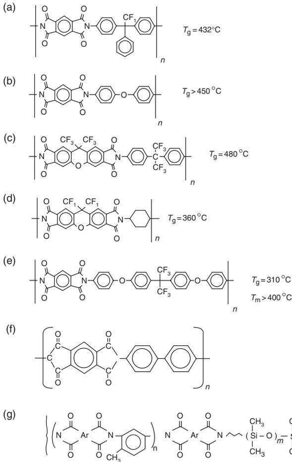
Fig. 6.9 Representative structures of: (a) PMDA/3FDA polyimide; (b) PMDA/ODA polyimide; (c) 6FXDA/6FDA polyimide; (d) 6FDACH polyimide, (e) PMDA/4-8DAF polyimide; (f) polyimide; (g) polyimide siloxane SIM™2010.
