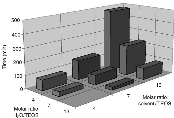
Fig. 8.12 Gelation time dependence on precursor composition.
