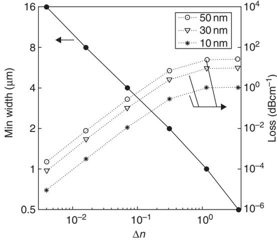
Fig. 11.11 Dependence of scattering loss on the index difference between core and cladding for a cladding index of 1.46; wavelength = 1550 nm; rms roughness of 10, 20, and 50 nm; and waveguide dimensions of  $1000 \text{ nm} \times 1000 \text{ nm}$  (right axis). If we set a maximum allowable loss of 1 dB/cm, then the minimum allowable waveguide dimension can be estimated (left axis).
