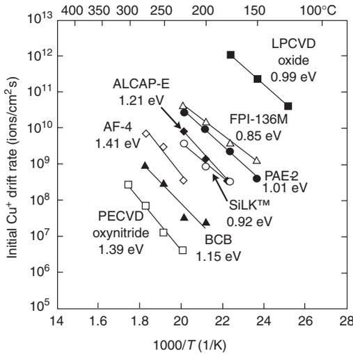
Fig. 9.30 Cu ion drift rate through a number of low- $\kappa$  and conventional dielectrics as a function of temperature. All were subjected to bias temperature stressing at a field strength of 1 MV/cm. The activation energies for each material are also given in the figure (adapted from Loke *et al.* [185] with permission). (© 1999 IEEE)
