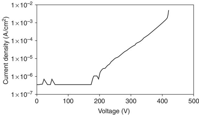
Fig. 8.28 Breakdown behaviour of aerogel thin films measured by mercury probe.
