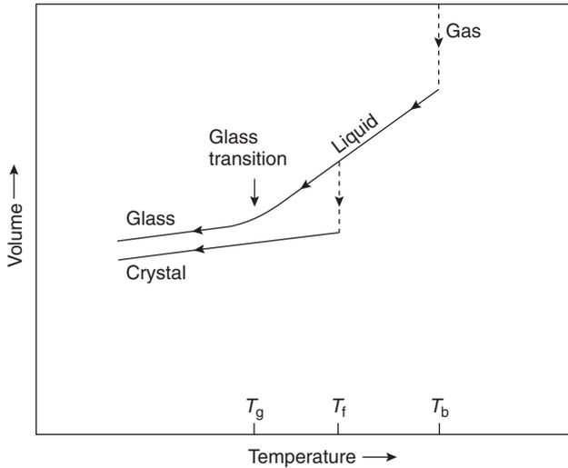
Fig. 6.3 A schematic plot of the volume of a material in various physical states as a function of the temperature (during cooling from high temperature). Transitions from vapor to liquid phase at  $T_b$  (boiling point), from liquid to a crystalline phase at  $T_f$  (the freezing point or melting point) during a very slow cool down, and from liquid to a glassy phase at  $T_g$  (the glass-transition temperature) during a fast cool down are shown.
