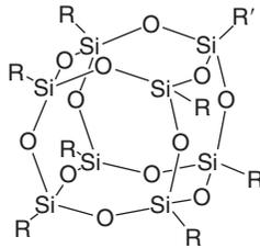
Fig. 9.6 An example of POSS monomer [52] (reprinted with permission).
