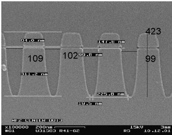
Fig. 4.5 STI structures using high-density plasma CVD oxide fill showing no delineation between trench oxide liner and fill.
