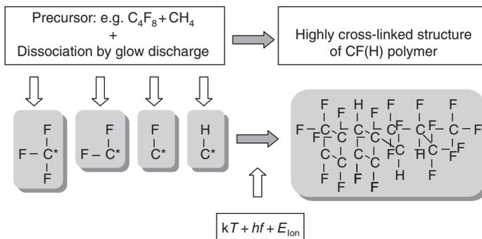
Fig. 7.3 Scheme of CF plasma polymerization process (PECVD).
