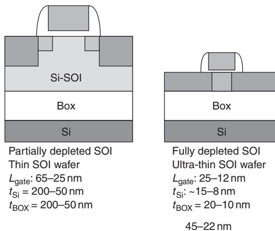
Fig. 13.12 SOI CMOS transistor structures.
