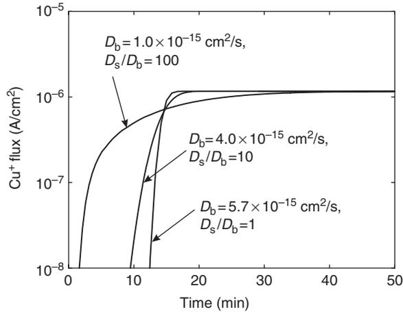
Fig. 9.42 Approach to steady-state of the cathode Cu<sup>+</sup> current flux ( $Pe = 2000$ ) [177, 205] (reprinted with permission).
