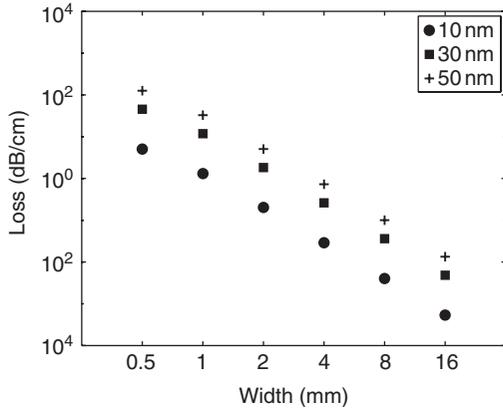
Fig. 11.9 Computed transmission loss in a polymer core waveguide plotted against waveguide width for various rms roughnesses. The core index is taken to be 1.52, the substrate index 1.46, and the cladding is air.
