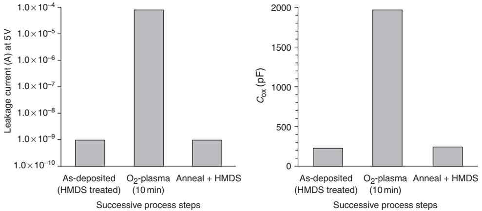
Fig. 8.32 Leakage current (left) and oxide capacitance (right) after deposition and additional O<sub>2</sub> plasma for resist stripping.
