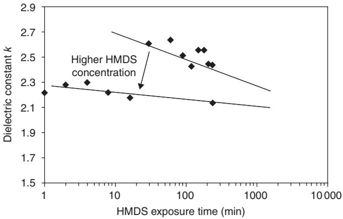
Fig. 8.21 Aerogel dielectric constant versus HMDS exposure time.
