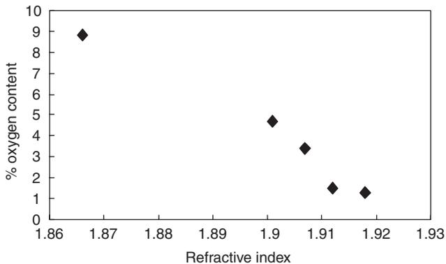
Fig. 5.13 A plot of correlation between oxygen content and refractive index of silicon nitride films.
