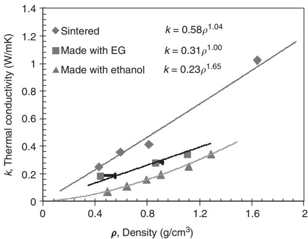
Fig. 9.22 Thermal conductivity of silica xerogel films as a function of density and process history [21] (reprinted with permission).
