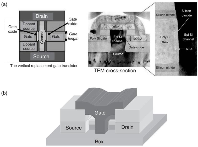
Fig. 13.14 Double gate CMOS vertical transistor: (a) vertical replacement gate (VRG) MOSFET; (b) double gate FinFET [29].
