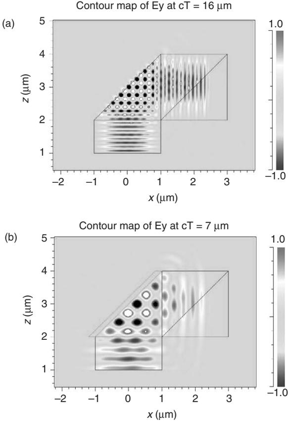
Fig. 11.2 Simulation of electric field intensity in a  $90^\circ$  bend mirror on a  $2\text{-}\mu\text{m}$  waveguide: (a) a high-index waveguide that uses a total internal reflection mirror; (b) a low-index waveguide that uses a metal mirror.
