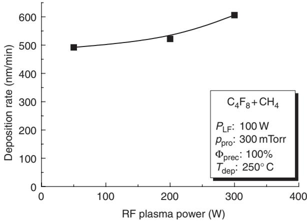
Fig. 7.7 Film deposition rate of CF polymers deposited at different RF plasma power.
