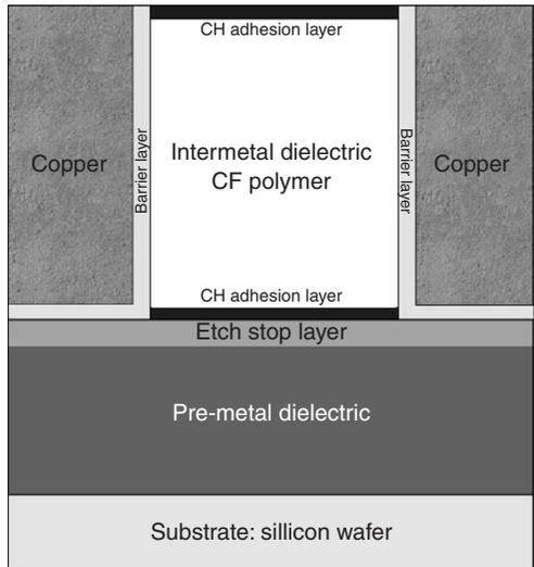
Fig. 7.16 Single damascene architecture for copper/low- $k$  (general description).
