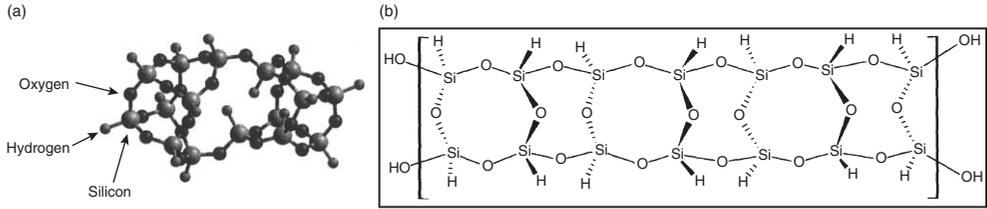
Fig. 8.1 Cage (a) and ladder (b) structure of HSQ as an example for the SSQs.
