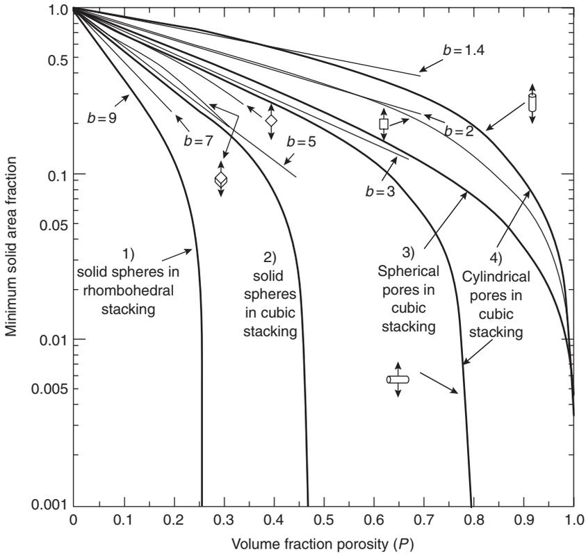
Fig. 9.14 Variation of the minimum solid area with porosity for idealized pores cubic stacking, Rice [82] (reprinted with permission).
