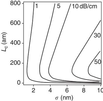
Fig. 11.10 Calculated contour map of loss with correlation length  $L_c$  and roughness  $\sigma$  as parameters. The index of the core is 3.5, the cross-section of the waveguide is  $500 \times 200$  nm, and the wavelength is 1540 nm (from [45]).
