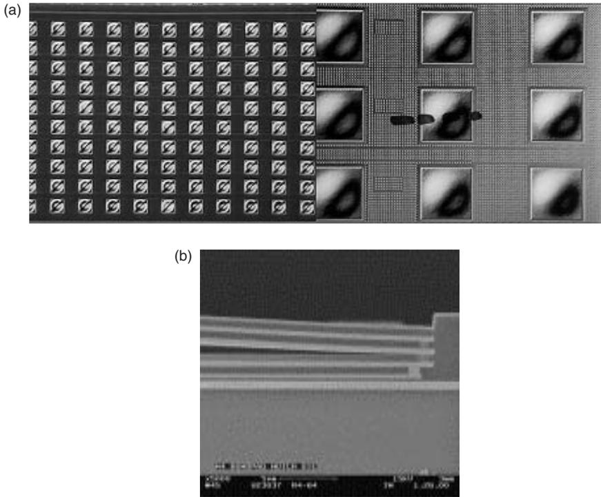
Fig. 4.7(a) Top-down image of delamination in unslotted probe pads. (b) SEM cross-sectional image of delamination at the Ta/FSG interface in an unslotted probe pad.
