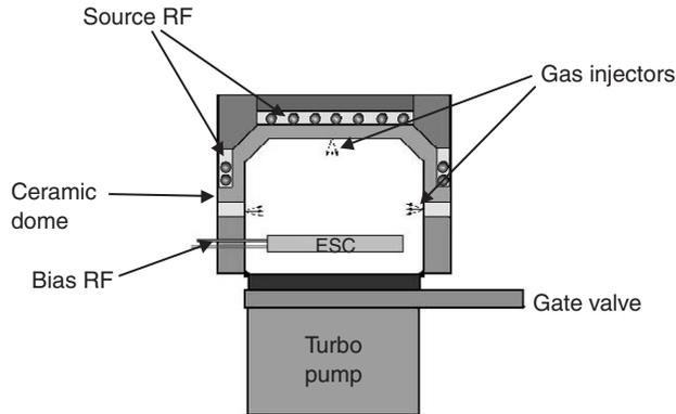
Fig. 5.5 Schematic of an HDPCVD chamber.
