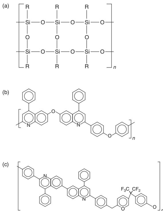
Fig. 6.4 Representative structures of: (a) hybrid organosiloxane (HOSP); (b) poly(quinoline)s; (c) poly(quinoline) (PQ)-100.
