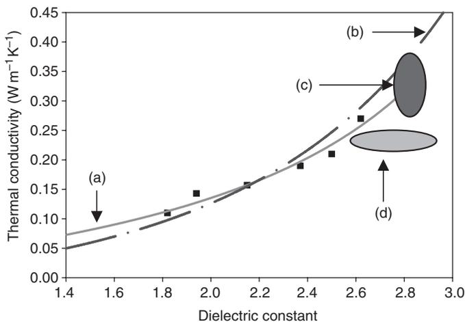
Fig. 3.17 Correlation of thermal conductivity and dielectric constant for low- $\kappa$  materials; symbol (■) represents the experimental data for porous MSQ films; curve (a) is for porous MSQ film and curve (b) for porous silica films; oval (c) includes various fully dense OSG materials and (d) includes various fully dense low- $\kappa$  polymers.
