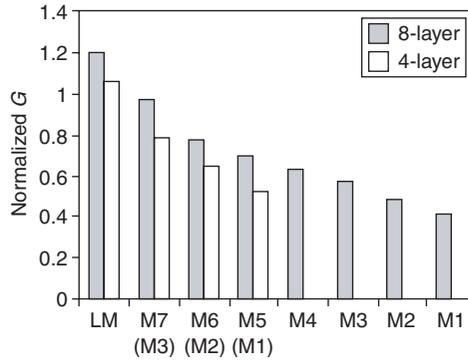
Fig. 4.11 Modeling results of crack driving force at the low-κ/passivation interface for a four-level stack versus an eight-level stack.
