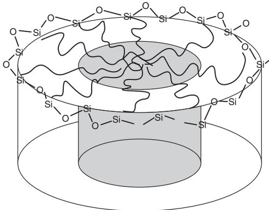
Fig. 8.8 Self-assembly of surfactants and soluble silica.
