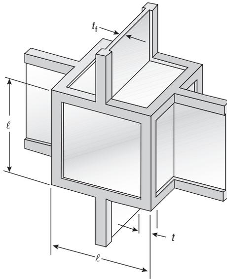
Fig. 9.12 Unit cell structure of a closed cell foam material [80] (reprinted with permission).
