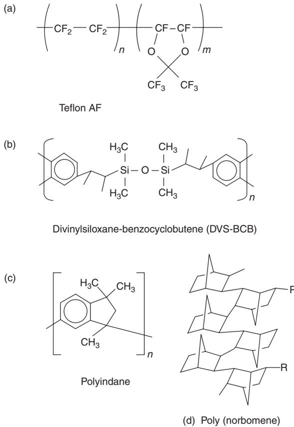
Fig. 6.6 Representative structures of: (a) Teflon AF; (b) divinylsiloxane-benzocyclobutene (DVS-BCB); (c) polyindane; (d) poly (norbomene).
