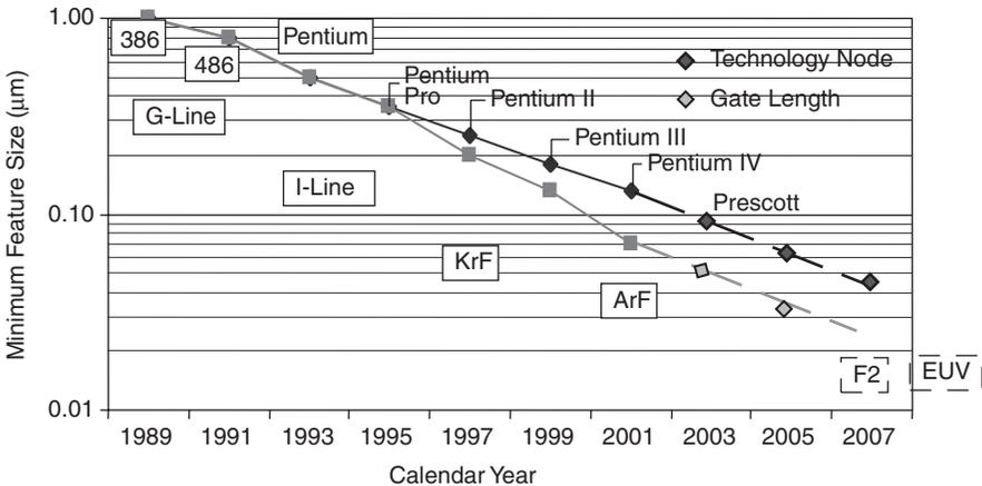
Fig. 13.2 Lithography-enabled feature size and gate length shrink for each technology node with time.
