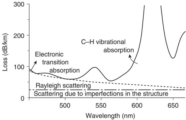
Fig. 11.7 Optical absorption coefficient plotted as a function of wavelength for PMMA [35].
