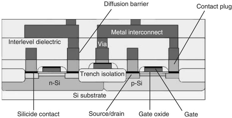
Fig. 1.2 Schematic drawing of a CMOS device.
