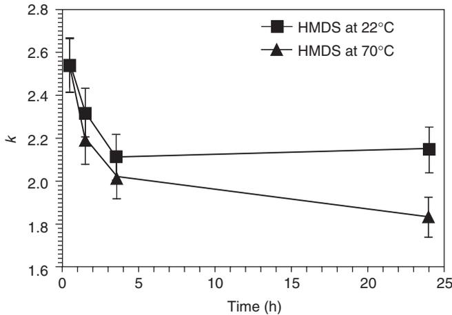
Fig. 8.23 Aerogel dielectric constant versus HMDS exposure time for different temperatures.
