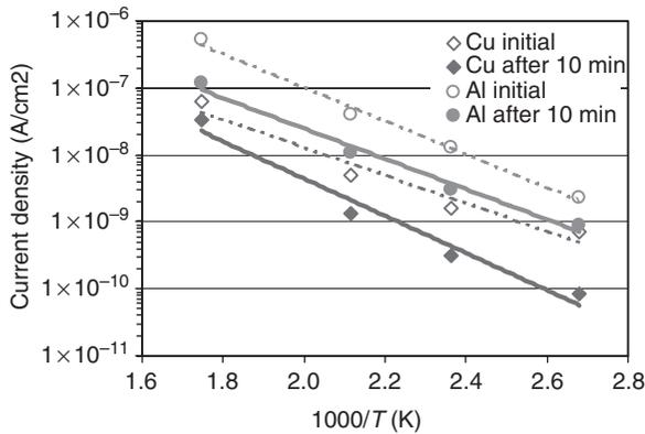
Fig. 9.33 Activation energy for copper and aluminum drift current through silica xerogel materials [177] (reprinted with permission).
