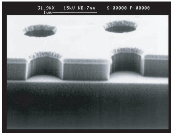
Fig. 7.18 Dry etched low-*k* polymer stack (hard mask on top, substrate silicon) [29] (© 2001 IEEE).
