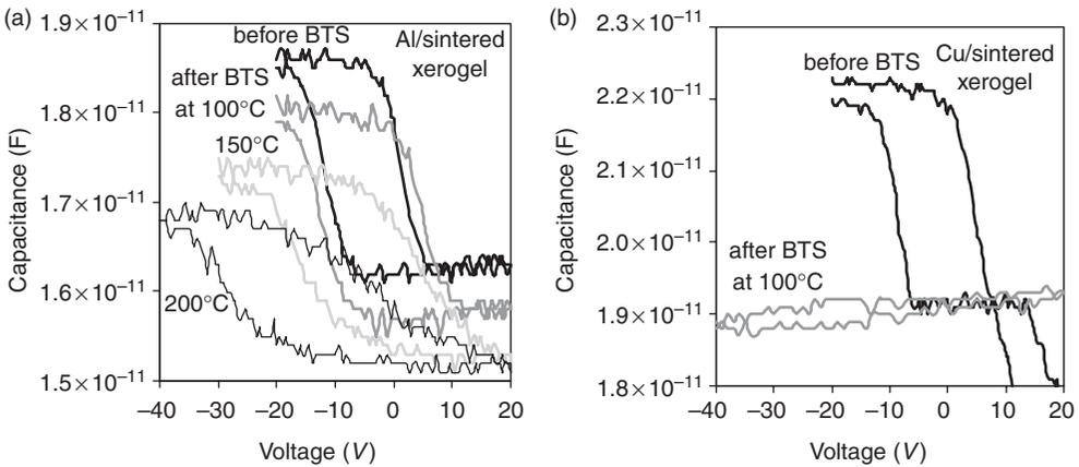
Fig. 9.37  $C$ - $V$  curve for xerogel film [177]. The  $C$ - $V$  curves and their corresponding  $I$ - $t$  curves during bias-temperature stressing are shown so that the current passed through the dielectric is known (reprinted with permission).
