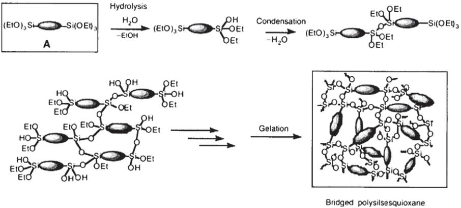
Fig. 9.5 Formation of bridged polysilsesquioxanes [51] (reprinted with permission).
