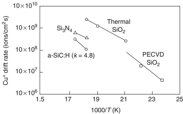
Fig. 9.29 Initial copper drift rate in a variety of inorganic, silicon-based dielectrics. Nitride and carbide dielectrics were stressed at a field strength of 2.8 MV/cm; thermal oxide was stressed at a field strength of 2 MV/cm and PECVD oxide at a field strength of 1 MV/cm (adapted with permission from Ref. [186]).
