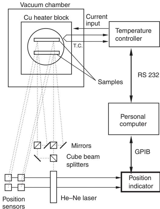
Fig. 3.3 Bending beam system for measuring thermal stress of thin films. Two beams can be measured simultaneously.
