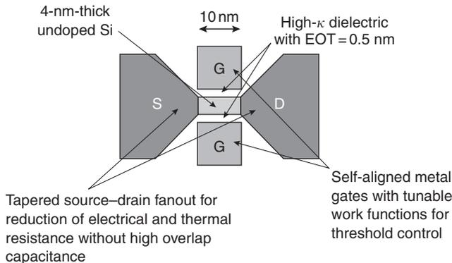
Fig. 13.13 The ultimate SOI transistor. (Source: Yuan Taur, UC San Diego, unpublished).
