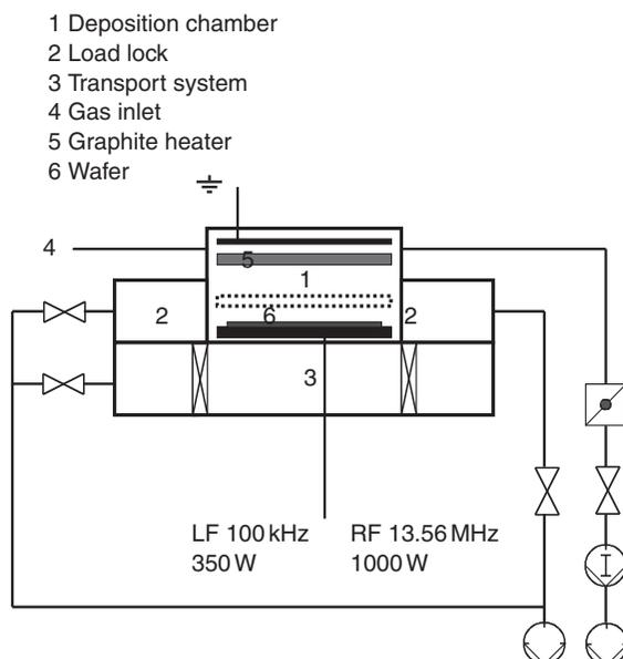
Fig. 7.4 Schematic of a commercially available etch tool (Tegal 1514e) used for CF polymer deposition, additionally equipped with heating system.
