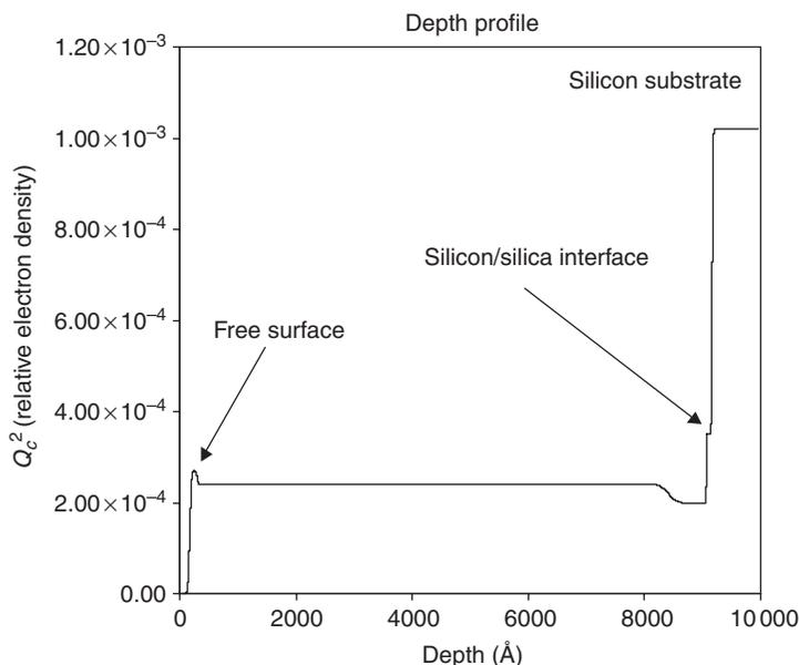
Fig. 3.9 The electron density space profile corresponding to the best fit to the data. At the free surface, a surface 'skin' about 5 nm thick with an electron density slightly higher than the bulk film is observed. A similar layer is observed at the film/silicon interface. The rest of the film has a uniform density.
