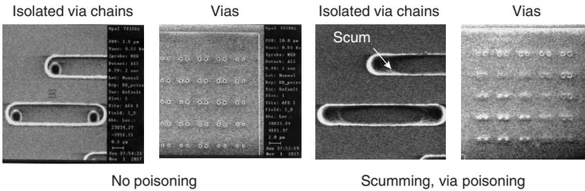
Fig. 5.28 Examples of with and without via poisoning.
