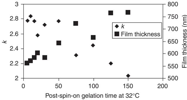
Fig. 8.18 Dielectric constant and film thickness for different post-spin-on gelation times.
