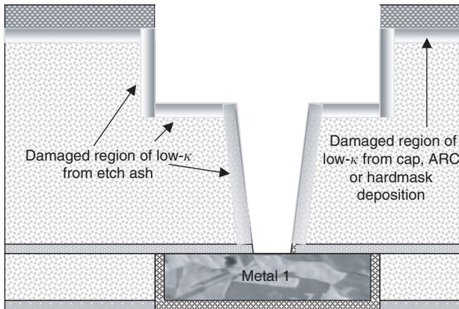
Fig. 4.4 Drawing of dual inlaid metal and via after etch and photoresist strip, showing regions where low- $\kappa$  surface has been altered.
