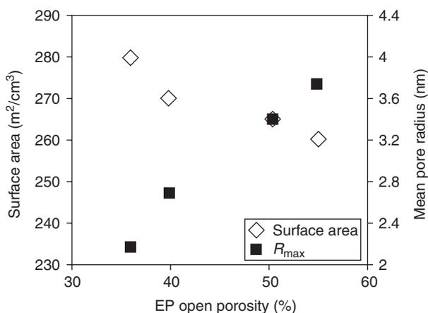
Fig. 8.27 Inner surface area and mean pore radius versus porosity measured by EP [27].
