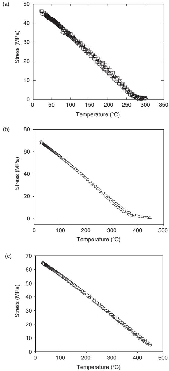
Fig. 3.13 Thermal stress measurement of (a) uncrosslinked, (b) partially crosslinked, and (c) fully crosslinked PAE film, showing an increase in the  $T_g$  from 275 to  $> 450$  °C. A corresponding rise in  $\kappa$  from  $\sim 2.9$  to 3.1–3.2 was observed for these films.
