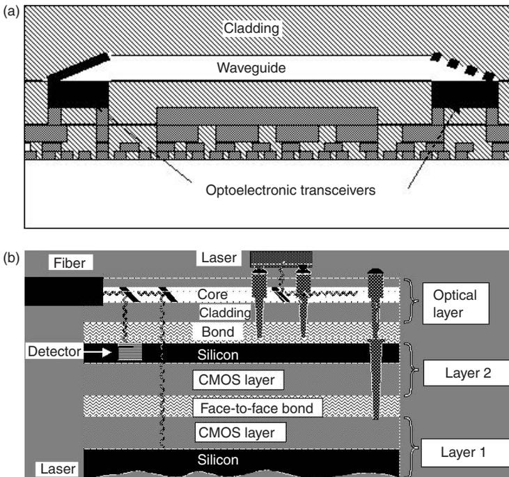
Figure 11.1 Schematics of various realizations of optical interconnects: (a) On-chip interconnects. As an example, the waveguide core would have a thickness of  $2\ \mu\text{m}$ , and each of the cladding layers would have thickness of a few micrometres as well. The optoelectronic transceiver dimensions would be of order a few micrometres on a side as well; (b) An example of three-dimensional, through-wafer interconnects based on the face-to-face architecture proposed by Gutmann *et al.* [4].
