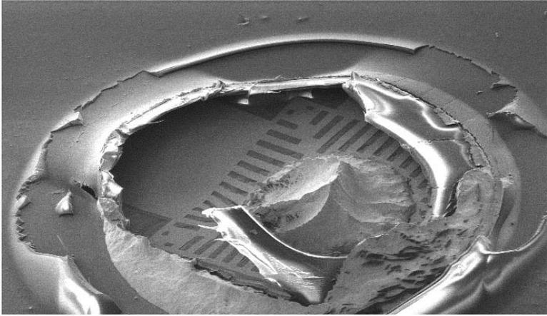
Fig. 4.14 FIB image of C4 BUMP die pull failures showing that the final passivation has delaminated from the Cu at the terminal metal level.
