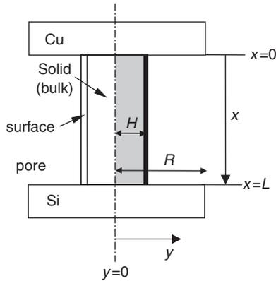
Fig. 9.38 Computational domain for diffusion through porous media [177].
