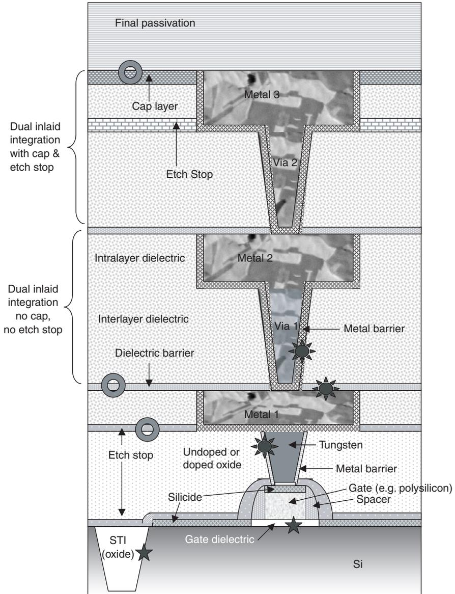
Fig. 4.1 Drawing of semiconductor device. ⊙, Denotes interfaces between dielectric materials; ★, denotes interfaces between metals and dielectrics; ★, denotes interfaces between dielectrics and semiconductors.
