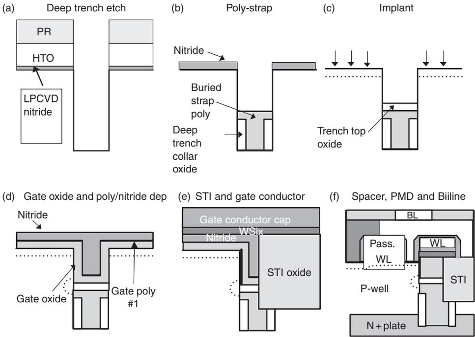
Fig. 5.21 Trench DRAM device fabrication steps.
