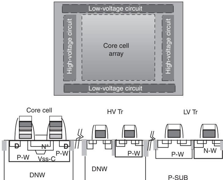
Fig. 13.8 Flash NOR transistor structure. It shows a flash core memory cell transistor structure that consists of the flash memory and the word line gate stack, with deep N-well, a high-voltage transistor, with deep N-well and the word line transistor, and a low-voltage transistor for logic circuits, which consists of conventional N- and P-wells, and polycide gate.
