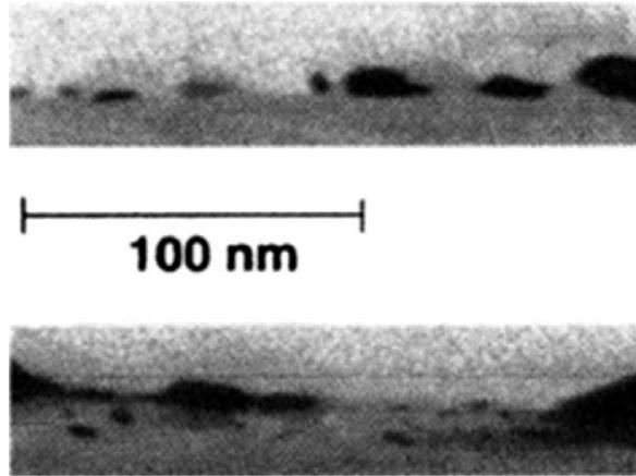
Fig. 9.32 TEM micrographs of Cu in Flare™. The upper figure shows clusters of Cu atoms on the surface of the polymer and the second shows Cu clusters within the polymer after heating for 12 h at 200°C (adapted from [189] with permission).
