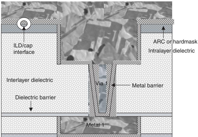
Fig. 4.2 Drawing of dual inlaid trench and via prior to CMP.
