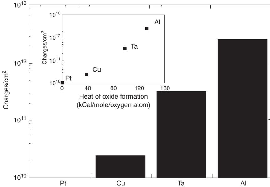
Fig. 6.13 Total number of charges after BTS at 150°C and 0.5 MV/cm for 30 min for all metal/HOSP/SiO<sub>2</sub>/Si capacitors. Inset shows relation of total charges to the heat of oxide formation per oxygen atoms. From Mallikarjuna *et al.* [55].
