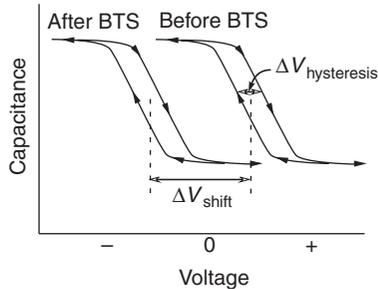
Fig. 9.35 Schematic diagram of a typical capacitance–voltage curve before and after bias-temperature-stressing injects ions into the dielectric.
