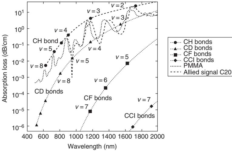
Fig. 11.8 Calculated absorption losses for various vibrational overtones [36].
