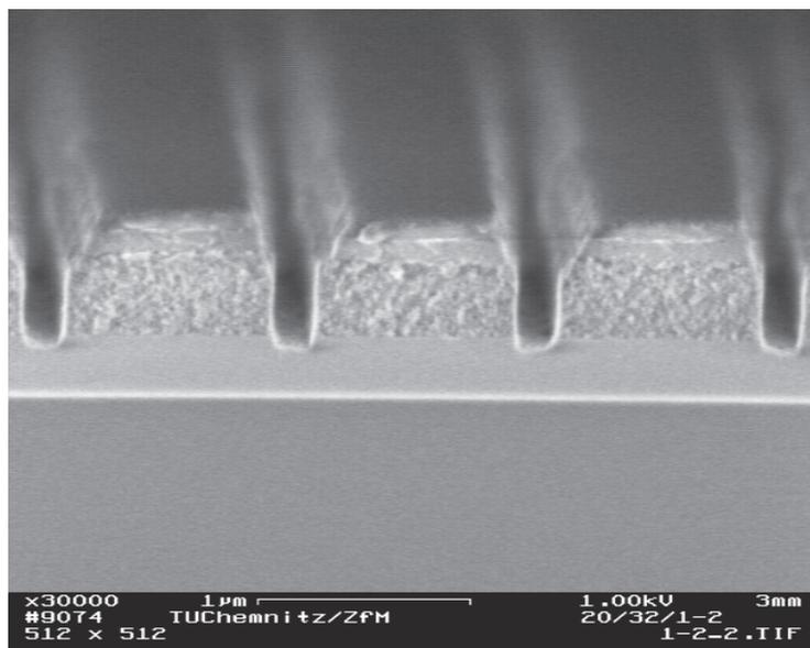
Fig. 8.36 Trenches (200 nm wide) etched into aerogel low- $k$  dielectric.
