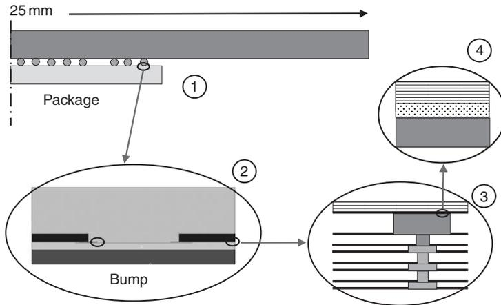
Fig. 4.13 Schematic diagram of the multi-level multi-scale submodeling technique used to evaluate the impact of the global packaging process on the local die-level structures.
