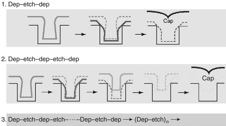
Fig. 5.4 Dep/etch concept of HDPCVD.
