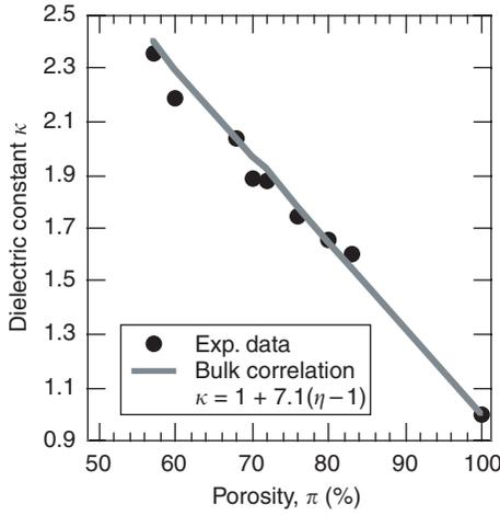
Fig. 9.7 Porosity correlation for xerogel film and comparison with Hrubesh correlation [60] (reprinted with permission).
