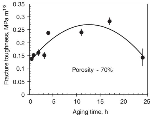
Fig. 9.18 Fracture toughness of xerogel films as a function of aging time [61] (reprinted with permission).
