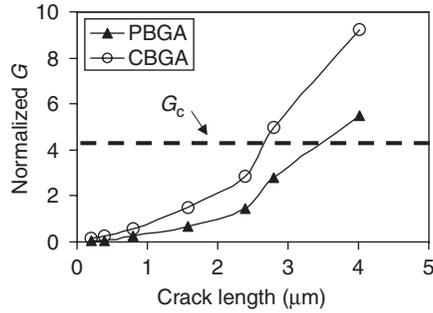
Fig. 4.8 Crack driving force versus crack length at the low- $\kappa$ /passivation interface.
