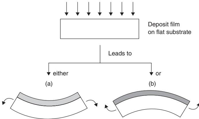
Fig. 2.4 Schematic representation of (a) tensile and (b) compressive stresses in the films deposited on a substrate. Arrows at the ends of film/substrate composites indicate tendency of the substrate to become flat (as it was before the film deposition).
