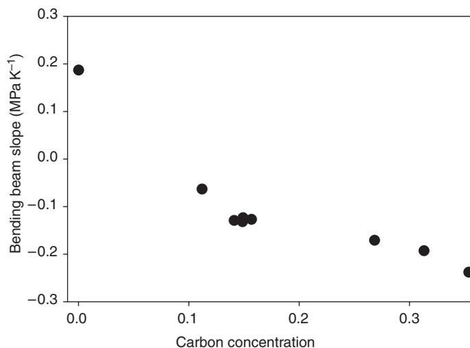
Fig. 3.15 Slopes ( $E \cdot \Delta\alpha$ ) of stresses vs. temperature for OSGs as function of carbon content (excluding H). TEOS is shown at 0% for comparison.
