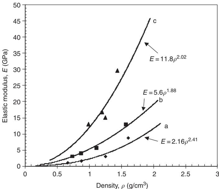
Fig. 9.16 Elastic modulus of films measured by nanoindentation; (a) films made with ethanol as the solvent; (b) films made with ethanol and ethylene glycol co-solvent mixture; (c) sintered films. Solid lines are power law fits [22] (reprinted with permission).
