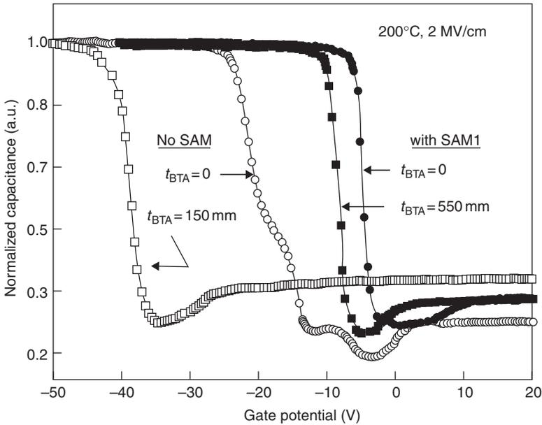
Fig. 6.14 Representative  $C$ - $V$  curves from a control sample (open legends) and a SAM1 coated MOS structure (filled legends) obtained prior to BTA (bias temperature annealing |equiv| bias temperature stressing) and after BTA at failure. From Krishnamoorthy *et al.* [138].
