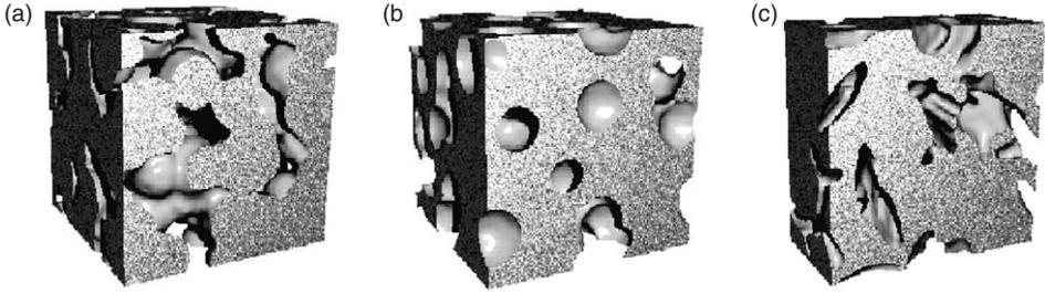
Fig. 9.15 Pieces of the various models studied by Roberts and Garboczi *et al.* [87]: (a) overlapping solid spheres; (b) overlapping spherical pores; and (c) overlapping ellipsoidal pores (reprinted with permission).
