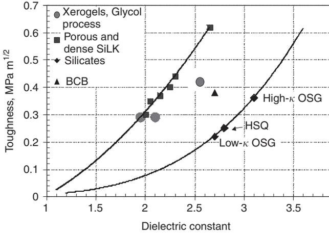
Fig. 9.21 Fracture toughness of various low-κ dielectric films measured by modified edge-lift-off test [61] (reprinted with permission).
