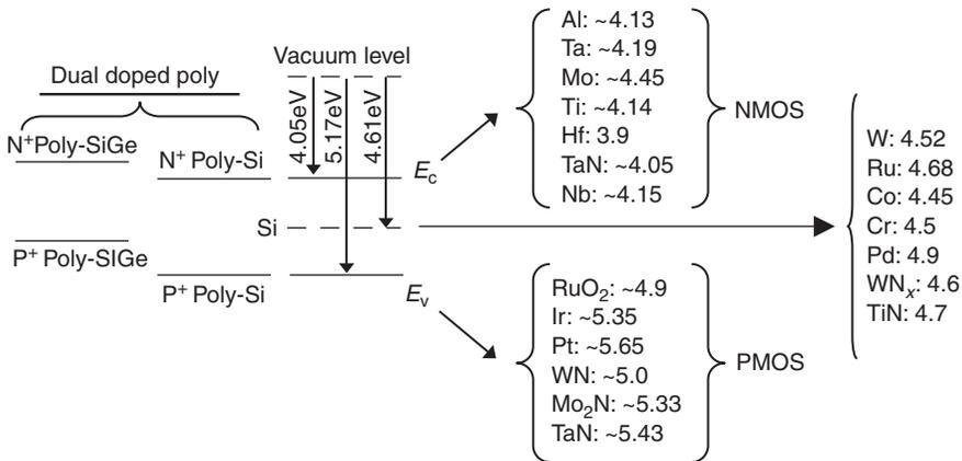
Fig. 13.6 Work functions of candidate gate electrodes.
