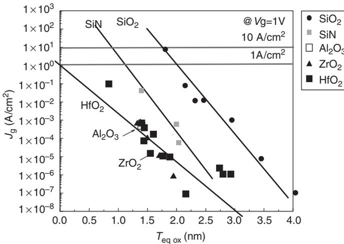
Fig. 13.5 Thickness dependence of leakage current for high- $\kappa$  materials.
