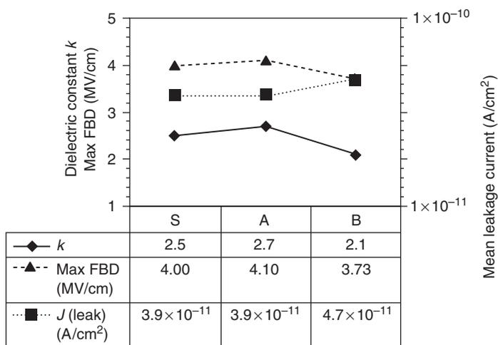
Fig. 8.13 Electrical parameters of aerogel films for application of different sol compositions.
