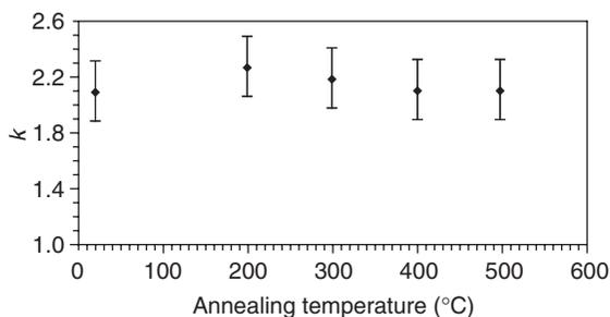
Fig. 8.30 Dielectric constant  $k$  of aerogel films at different vacuum annealing temperatures.
