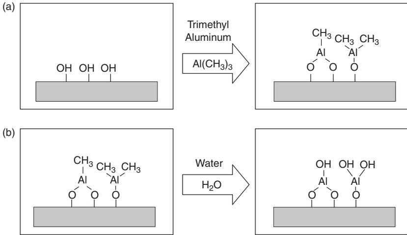
Fig. 10.2 Illustration of the two, sequential, self-limiting surface reactions that define Al<sub>2</sub>O<sub>3</sub> ALD.
