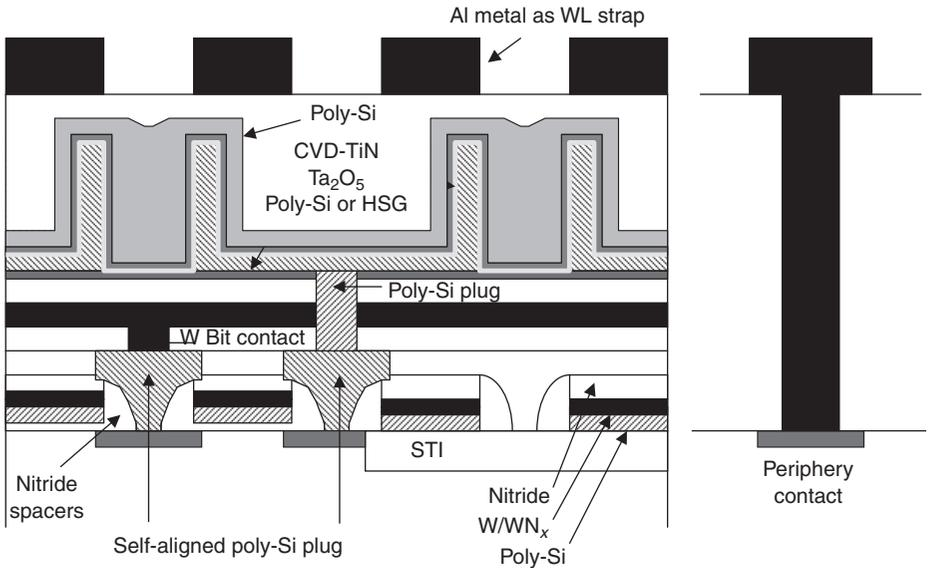
Fig. 13.7 DRAM cell and periphery contact structure.
