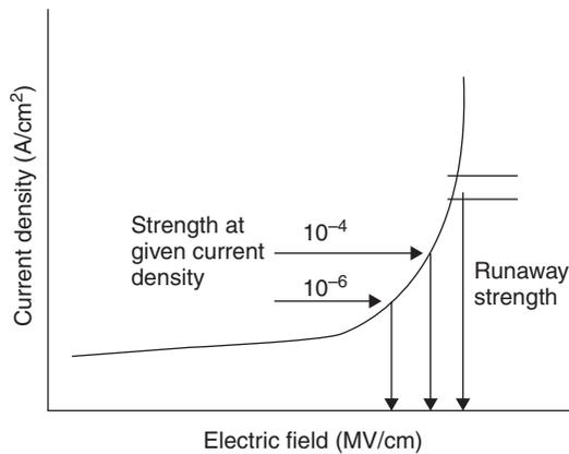
Fig. 2.1 Schematic representation of current density through a dielectric as a function of the applied field.
