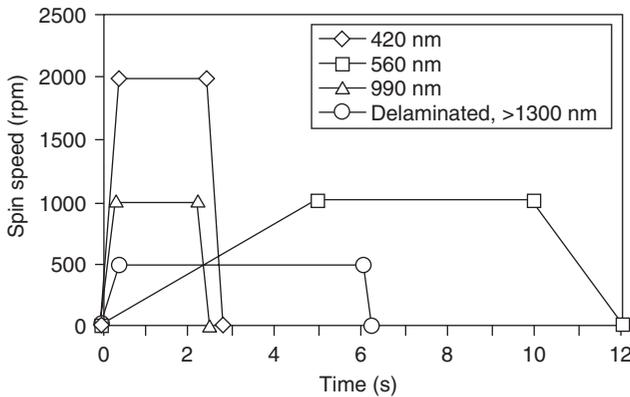
Fig. 8.16 Spin-on regimes and resulting thicknesses for aerogel sol-gel processing.
