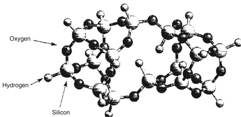
Fig. 9.4 A proposed structure of porous MSQ, *DendriGlass*<sup>TM</sup> [46] (reprinted with permission).
