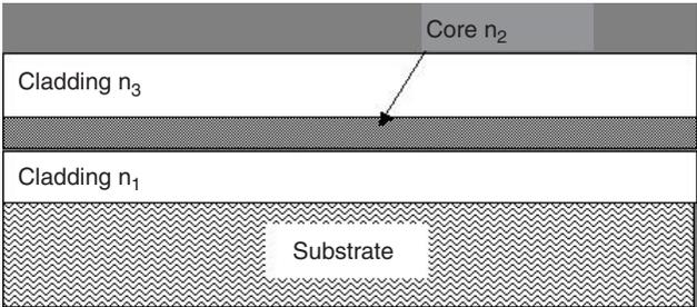
Fig. 11.3 Schematic of a prototypical three-layer index-difference waveguide.
