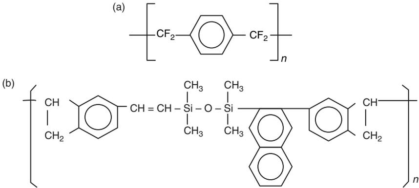
Fig. 9.3 (a) Structure of Parylene-F, (b) Structure of BCB [61].
