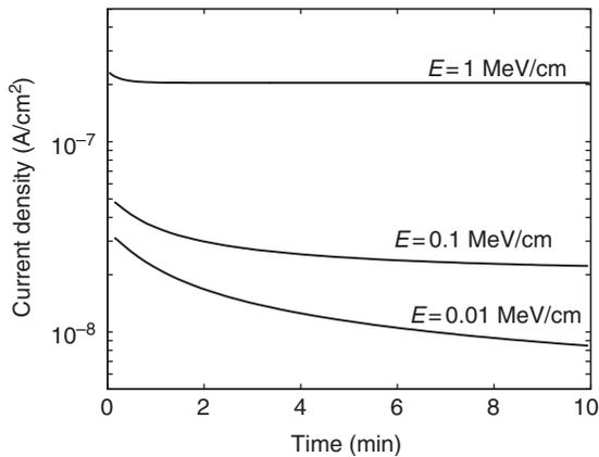
Fig. 9.40 Effect of electric field strength on the anode current for the system [177, 205] (reprinted with permission).
