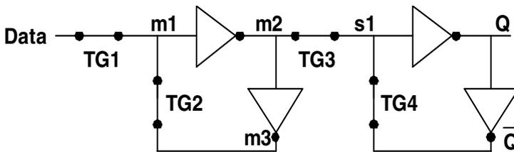
Figure 4-15. The equivalent circuit of the flip-flop.
