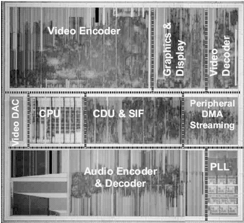
*Figure 1-5. A typical system on chip [17].*
