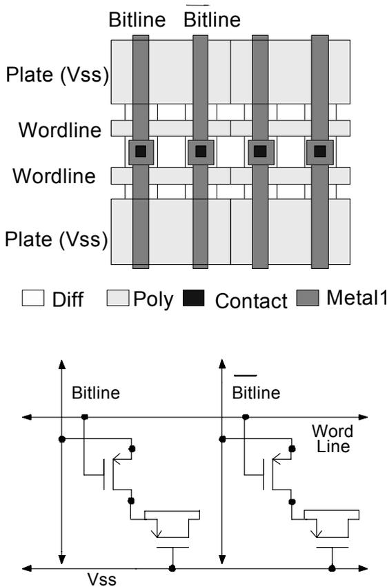
Figure 5-5. DRAM cell and the schematic.
