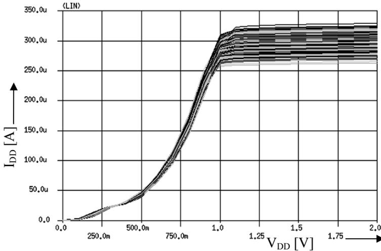
Figure 6-14. Amplifier current signatures with process spread.
