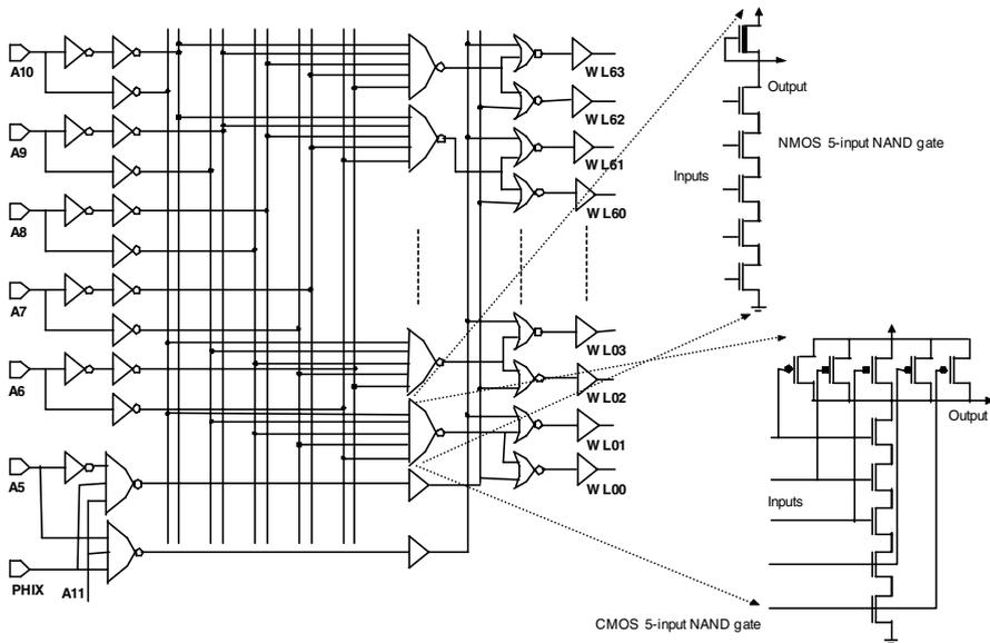
Figure 5-15. A typical RAM address decoder with implementations in NMOS and CMOS technologies.
