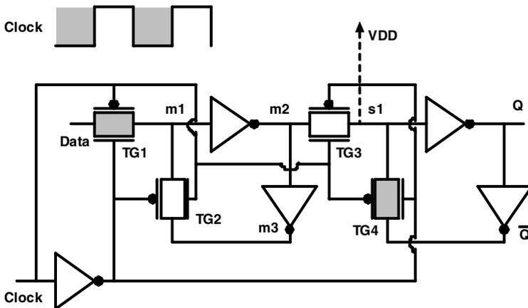
Figure 4-13. A bridging defect between  $s1$  and  $V_{DD}$  in a typical CMOS flip-flop is not detected by  $I_{DDQ}$ .
