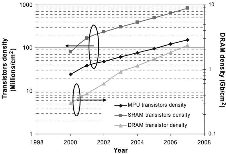
Figure 1-4. Growing transistor density [22].
