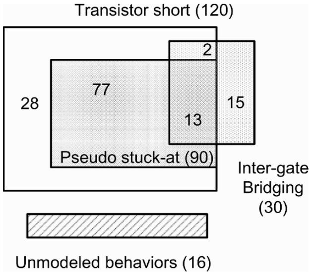
Figure 4-11. Overlap of faulty behaviours observed by Aitken [1].
