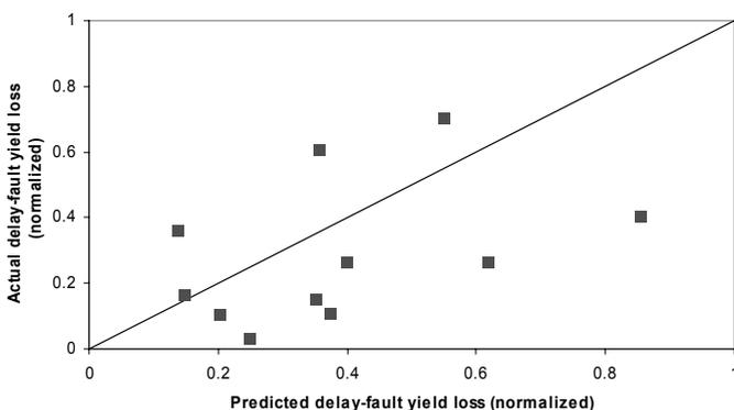
Figure 2-17. Correlation of predicted and actual normalized yield loss due to delay faults.
