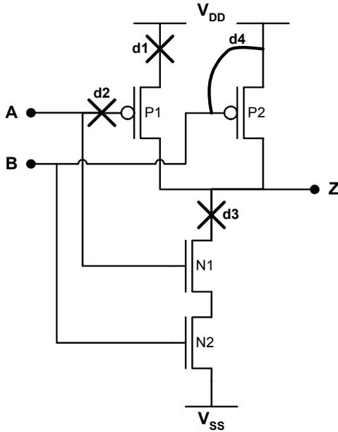
Figure 3-6. Open and bridging defects causing SOP behavior.
