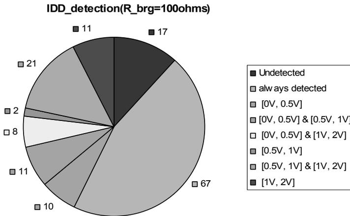
Figure 6-19. Number of detected faults per  $V_{DD}$  interval.
