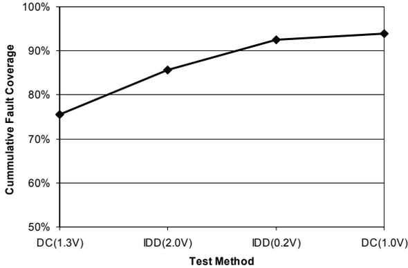
*Figure 6-23. Optimized set of only structural tests.*
