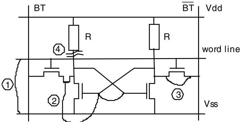
Figure 5-2. Examples of defects for different fault classes.
