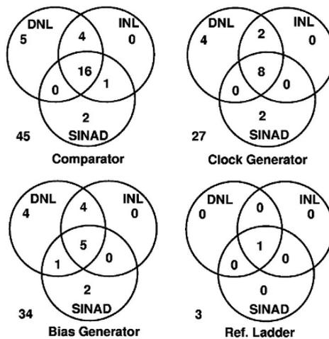
Figure 6-33. Fault detection capabilities of different tests.
