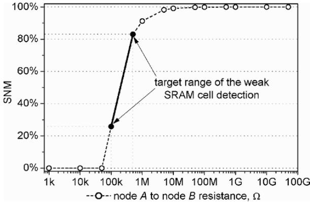
Figure 5-33. SNM range to be modeled by the weak fault model.
