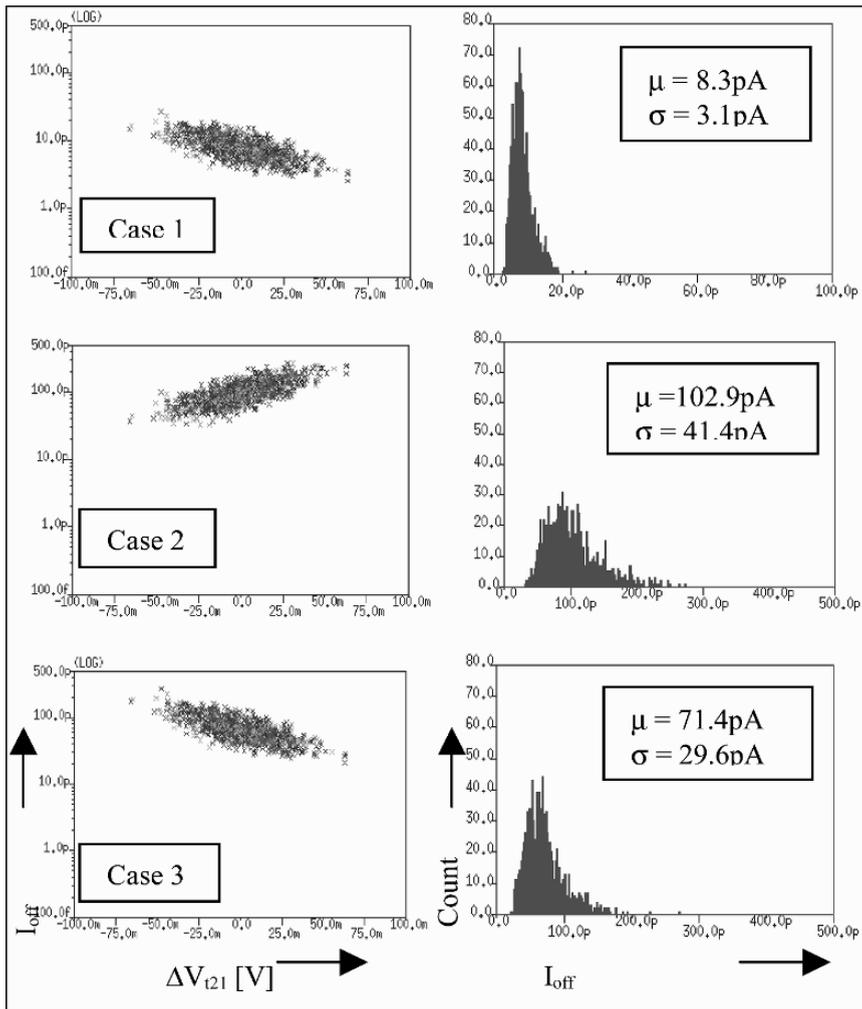
Figure 2-6. Monte Carlo simulations to estimate intra-die off-state current. Scatter plots present points for off-state current vs.  $V_i$  mismatch. Histograms show the corresponding distribution of off-state currents.
