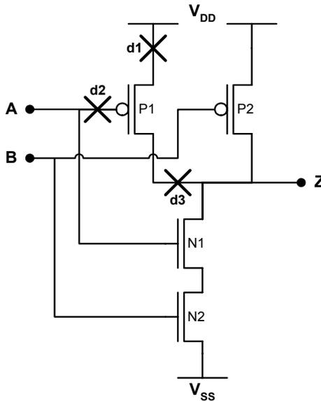
Figure 3-4. Undetected open defects in a 20input CMOS NAND gate by SAF test vectors.
