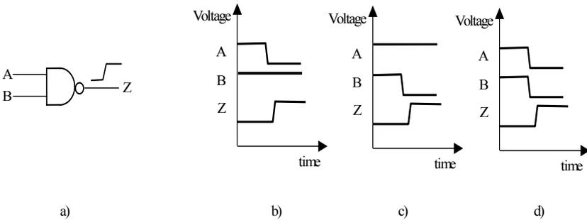
Figure 2-8. Input combinations to create a low-to-high transition at the output of a 2-input NAND gate.
