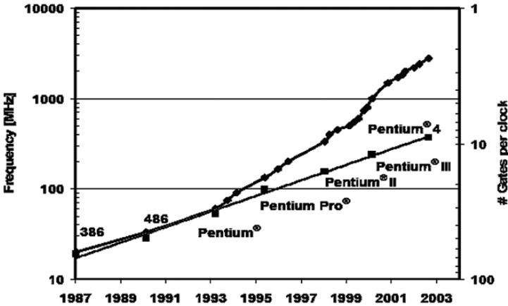
Figure 3-12. Frequency and gate delay with technology scaling [109].
