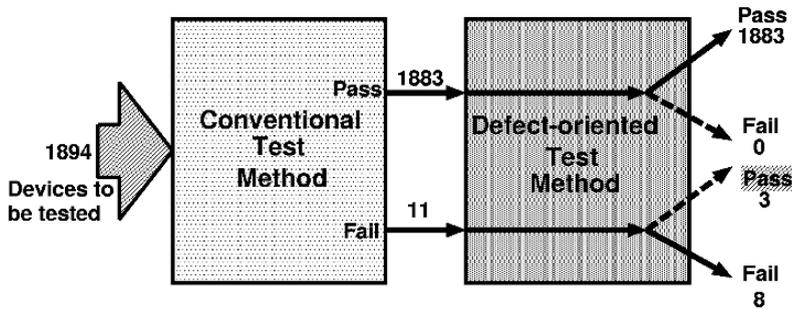
Figure 6-10. The results of the second experiment over the Class AB amplifier.
