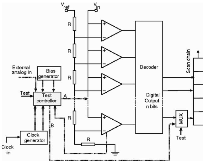
Figure 6-37. A full flash A/D converter block diagram with DfT features.
