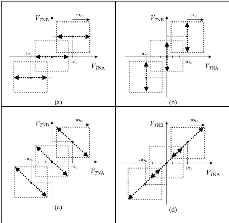
Figure 2-12.  $V_t$  mismatch analysis. (a) constant  $V_{INB}$ , (b) constant  $V_{INA}$ , (c)  $V_{INA}$  and  $V_{INB}$  running in opposite directions, (d)  $V_{INA}$  and  $V_{INB}$  running in the same direction.
