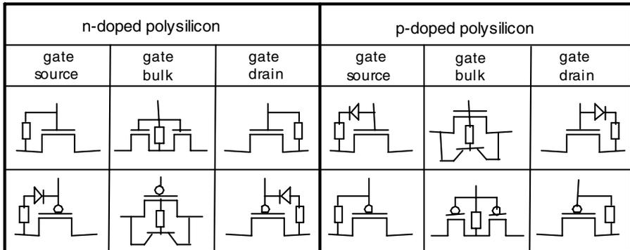
Figure 4-7. A generalized gate oxide defect model [39].
