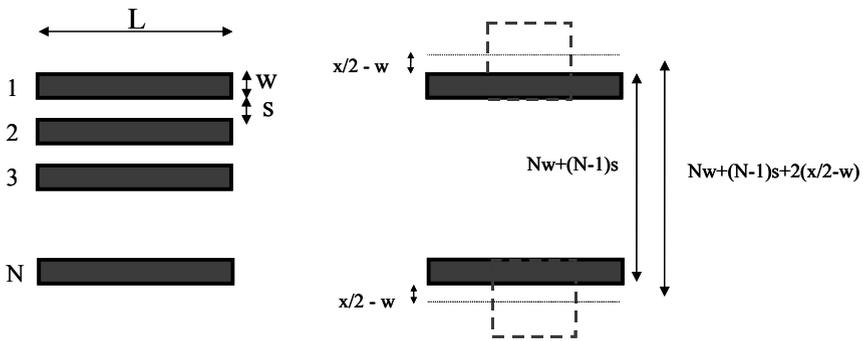
Figure 2-29. Setup to find the critical area of  $N$  conductors.
