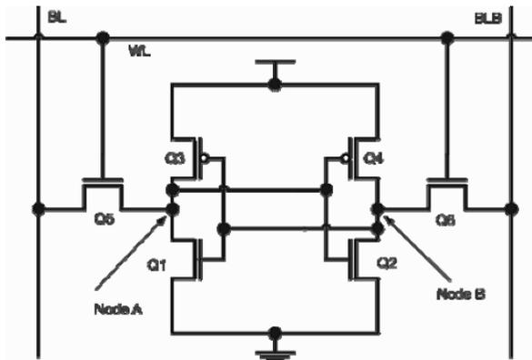
Figure 5-24. The 6T SRAM cell.
