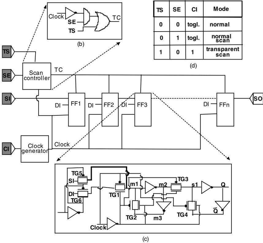
Figure 4-17. Transparent scan with single clock (a), scan controller logic diagram (b), modified scan flip-flop to facilitate single clock test mode operation (c), and flip-flop operational modes (d).
