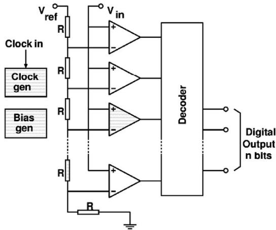
Figure 6-32. Block diagram of a flash A/D converter.
