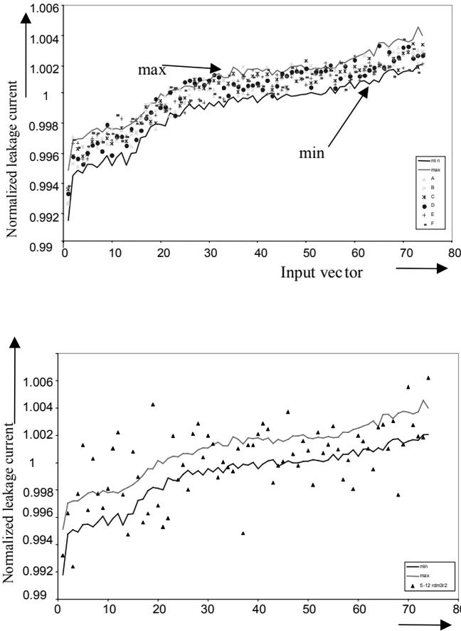
Figure 2-7. Impact of intra-die variations on leakage current. (a) expected correct behavior (b) intra-die variations of DSPs with leakage out of the tolerance window.
