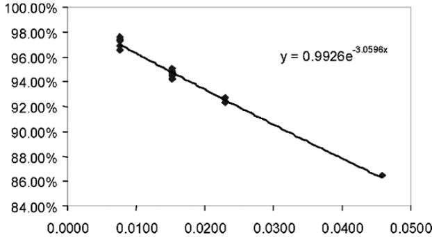
Figure 7-8. Fitting yield measurements to Poisson distribution.
