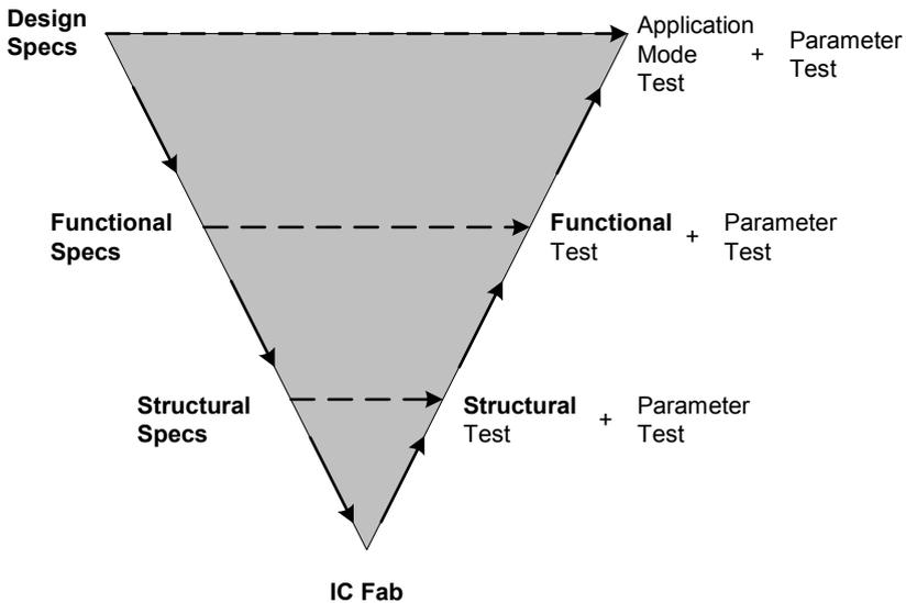
Figure 3-1. An idealized design and verification process [7].
