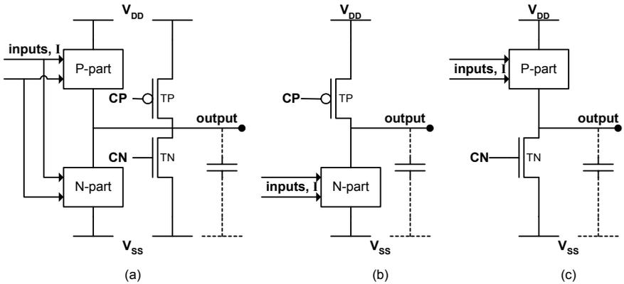
Figure 3-9. Single pattern SOP fault detection procedure.
