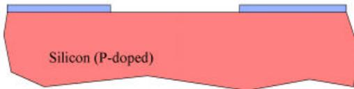
Fig. 1-6: The oxide is etched away and the photoresist is removed.
