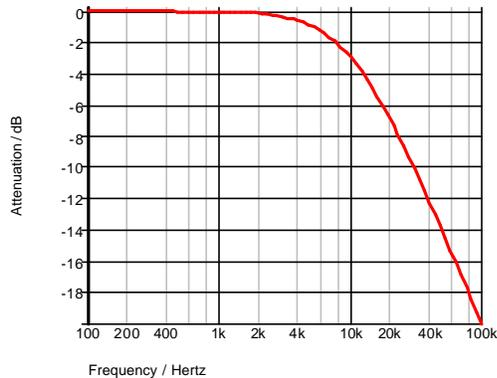
Fig. 13-2: Frequency response of single-pole filter.
