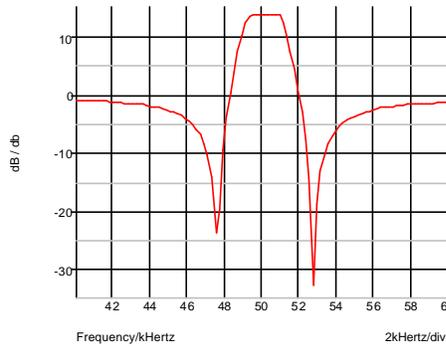
Fig. 13-19: Response of a fourth-order elliptic band-pass filter.
