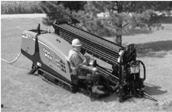
**FIGURE 4.6** Directional drilling machine [DitchWitch].
