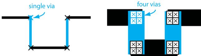
*Figure 8–3. Thicker wire allows additional vias between metals.*
