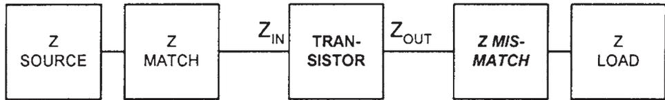
Figure 3.48 Selective output mismatching of an active device to lower stage gain.
