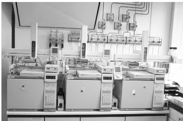
FIG. 12. Picture of optimized unit for ee determination based on three GC instruments driven by one PC (104).
