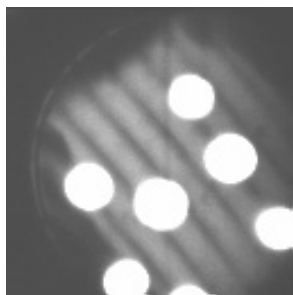
Fig. 5.93 Result of placing the detector in a conjugate sample plane. The dynode structure, in this case of a H5773, appears in the image. The bright circles are fluorescing beads in the sample
