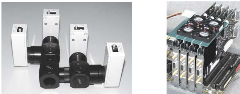
Fig. 5.83 Four-PMT detector assembly ( left ) and four-channel TCSPC imaging system ( right , on a Pentium motherboard)
