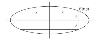
Let (x, y) represent the point P in the first quadrant where the rectangle meets the ellipse. Then the dimensions of the rectangle are 2x by 2y so its area A = 4xy. Since P lies on the ellipse, its coordinates must satisfy the equation of the ellipse,  $\frac{x^2}{200} + \frac{y^2}{50} = 1$ . We solve for y:
