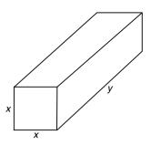
$V=x^2y$ . The postal restrictions say that 4x+y cannot exceed 108 inches. For maximum volume we take 4x+y=108. Equivalently, y=108-4x and  $0 \le x \le 27$ . (If x>27, y<0.)
