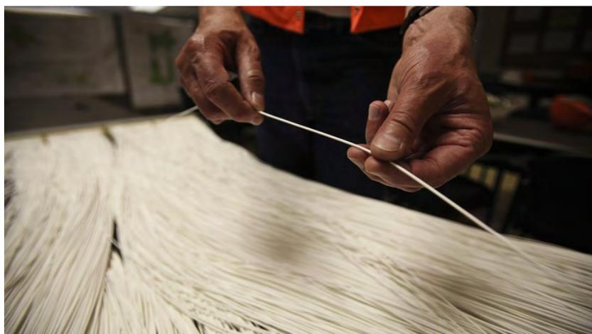
**Figure 2.2** hollow fiber membranes
