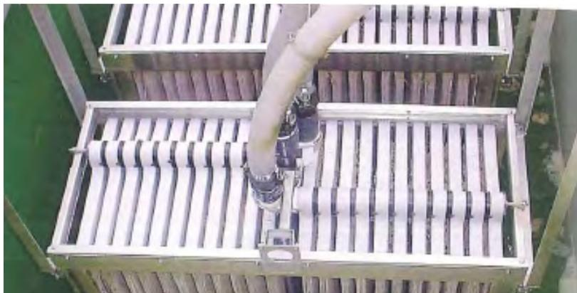
**Figure 8.7** module cassettes during In-air cleaning
